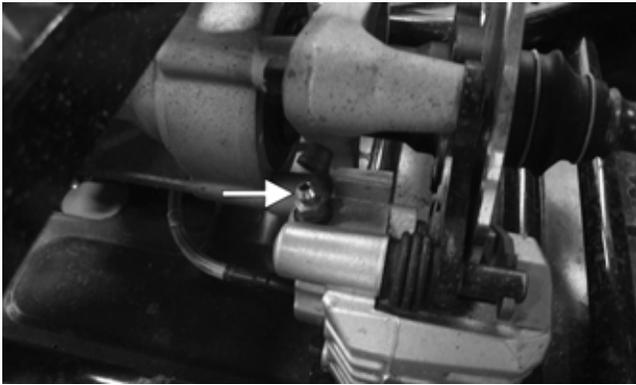
■NOTE: During the bleeding procedure, watch the reservoir very closely to make sure there is always a sufficient amount of brake fluid. When the level falls below MIN, refill the reservoir before the bleeding procedure is continued. Failure to maintain a sufficient amount of fluid in the reservoir will result in air in the system.
