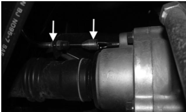
13. Remove the cap screws from the drive coupler flange; then remove the upper and lower mounting cap screws and remove the differential from the frame.
