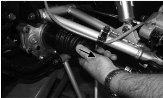
■NOTE: In some instances it may be necessary to use a pry-bar between the gear case housing and axle coupler shoulder to dislodge the splines.
