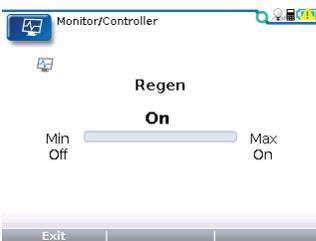
“Regen” shows regenerative braking and activates when the brake pedal is pressed. Regen deactivates when the pedal is released.
