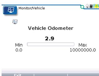
“Vehicle Odometer” indicates vehicle distance traveled in units of miles. For accurate distance measurements, the speed to RPM parameters must be set correctly.
