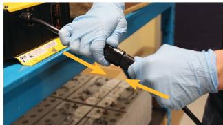
Figure 3: Reconnect AC power to the charger.
