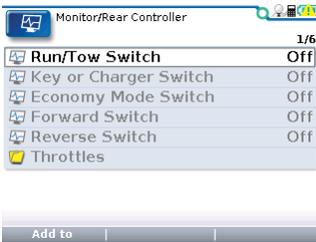
“Rear Controller” allows access to a sub menu to see rear controller inputs. The front controller is a SLAVE controller, and is controlled by the rear controller.
