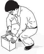
**The batteries must be removed before any service or repairs that can cause sparks.**
