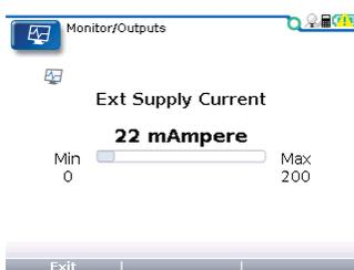
“Ext. Supply Current” shows the combined current of the external + 12 volt and + 5 volt supplies (pins 25 and 26)
