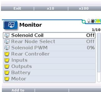
The "Monitor" menu selection shows controller functions, inputs, and outputs.
