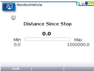
“Distance Since Stop” shows the distance traveled by the vehicle starting from a stop. In effect, the vehicle is used as a tape measure. In other words if you travel 300 feet in forward and then 300 feet in reverse the distance would be 600 feet. The distance is continuously updated and will stop and restart when motor RPM = 0
