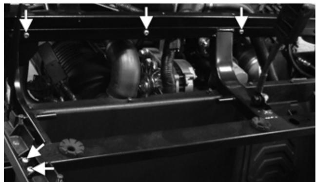
2. Reinstall the behind-the-seat storage box panel; then reinstall the rear side panels and rear inner fenders; then reinstall the rear seats.
