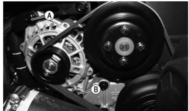
4. Remove the adjuster cap screw and pivot bolt and remove the alternator.
