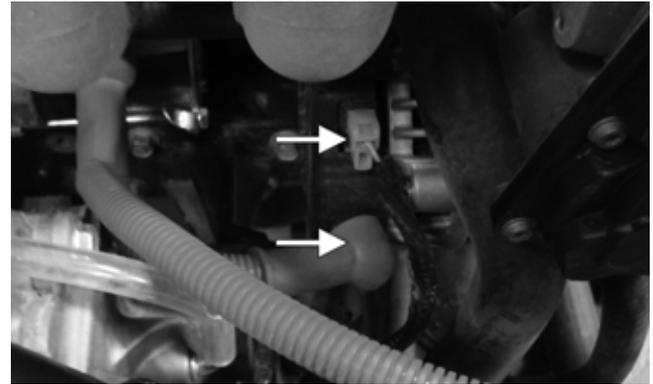
3. Loosen the alternator adjuster cap screw (A) and the pivot bolt (B); then remove the serpentine belt.
