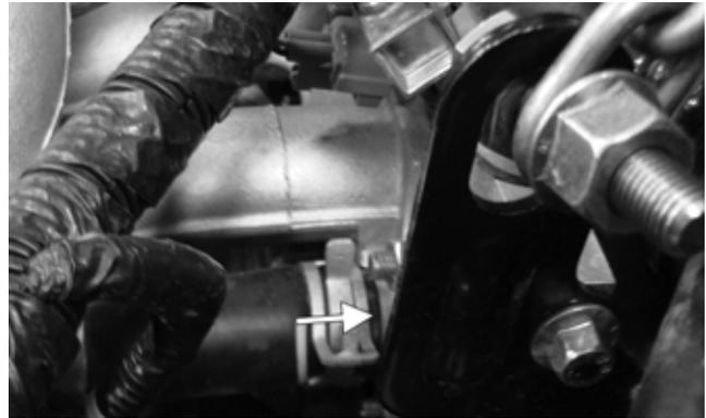
15. Remove the suitable clamps that were used to minimize coolant leakage.
