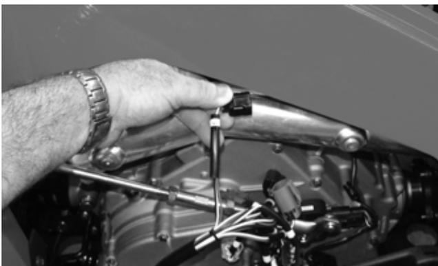
3. Using a multimeter, connect the black tester lead to the black socket (GND) on the analyzer and the red tester lead to the white socket (VAR); then select the DC Voltage position. With the vehicle off, the gauge should read 0.58-0.62 and at Wide-Open Throttle it should read up to approximately 3.7.
