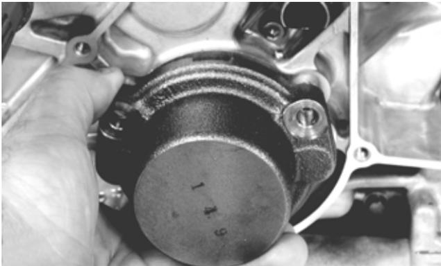
12. Remove the snap ring securing the oil pump driven gear (A); then remove the gear noting the direction of the sides of the gear for installing purposes. Account for a pin and a washer.
