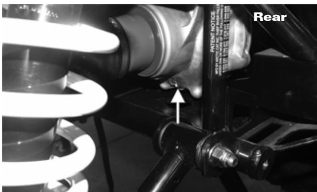
4. After all the oil has been drained, install the drain plugs and tighten securely.
