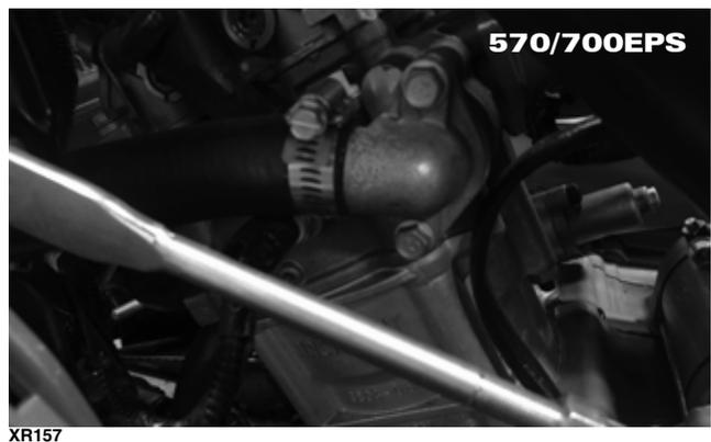
5. Install the exhaust pipe using a new seal at the cylinder head and loosely install the retaining cap screws; then install the muffler with a new GRAFOIL seal and secure with two springs. Tighten the exhaust pipe retainer cap screws to 20 ft-lb.
