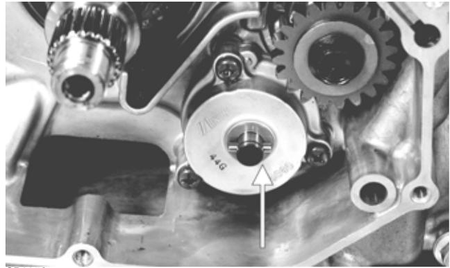
13. Using an impact driver, remove the three Torx-head screws securing the oil pump; then remove the pump.
