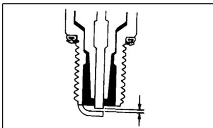
When installing the spark plug, be sure to tighten it securely. A new spark plug should be tightened 1/2 turn once the washer contacts the cylinder head. A used spark plug should be tightened 1/8-1/4 turn once the washer contacts the cylinder head.
