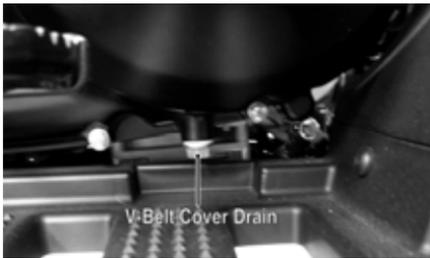
■ **NOTE:** If the ATV has been driven through water, the V-belt cover must be drained of any water.
