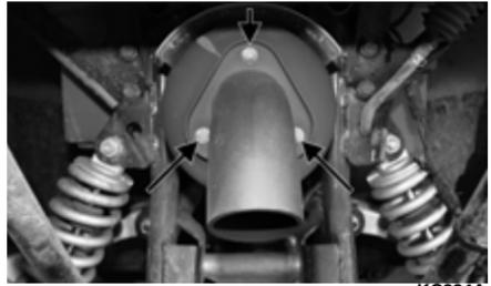
2. Using a suitable brush, clean the carbon deposits from the screen taking care not to damage the screen.
