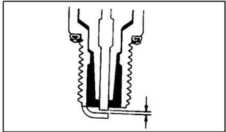
When installing the spark plug, be sure to tighten it securely. A new spark plug should be tightened 1/2 turn once the washer contacts the cylinder head. A used spark plug should be tightened 1/8-1/4 turn once the washer contacts the cylinder head.
