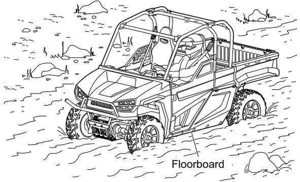
**⚠ WARNING** Deep or fast-flowing water can cause loss of vehicle control and lead to possible injury or death. Never cross water that is deeper than the bottom of the floorboard.
