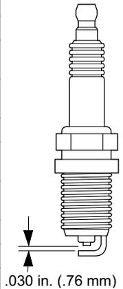
3. Apply a light coat of anti-seize compound to the spark plug threads.
