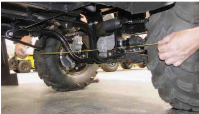
Fig. 15 Wheel Alignment Rear of Front Tires
