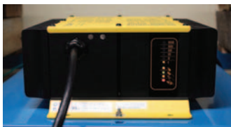
Figure 4: Charger LED indicator self-test.
