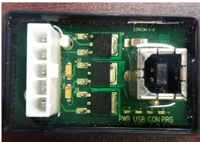
Fig. 6 USB Communication Module with LED indicators on Bottom Right
