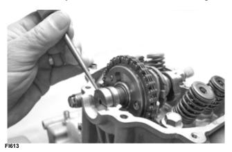
**NOTE:** Care should be taken not to drop the C-ring down into the crankcase.
