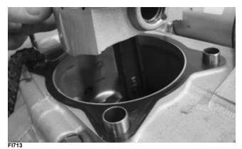
3. Lubricate the inside wall of the cylinder; then using a ring compressor or the fingers, compress the rings and slide the cylinder over the piston. Route the cam chain up through the cylinder cam chain housing; then remove the piston holder and seat the cylinder firmly on the crankcase.
