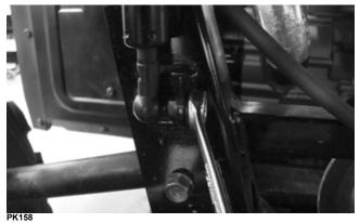
3. Remove the retaining clips from each clevis pin; then remove both pivot pins.
