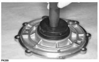
3. Place the pinion gear shim into position; then, using a set of press blocks, press the pinion gear into a new bearing.
