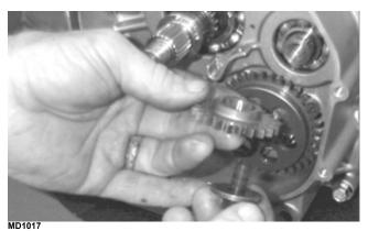
16. Remove the snap ring holding the oil pump driven gear.
