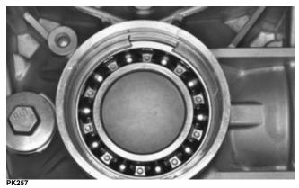
12. Using a bearing driver, remove the case side bearing from the inside of the case.
