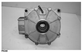
5. Remove the ring gear from the housing. Account for the housing side shim.
