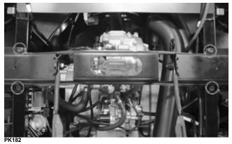
15. From each side of the vehicle, loosely install the eight cap screws securing the outside of the seat frame to the top of the main frame.
