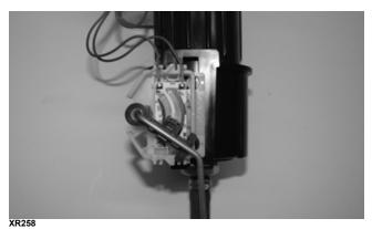
5. Connect the blue wires using the supplied splice connectors from the fuel level sensor kit. Secure the wires.
