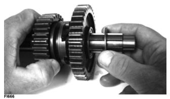
4. Place the reverse driven bushing (13) onto the shaft; then install the bearing (14), gear (15), and splined washer (16). Secure with a snap-ring.
