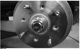
9. Secure the brake line to the knuckle; then secure the brake caliper to the knuckle with the two new "patch-lock" cap screws. Tighten to 20 ft-lb.
