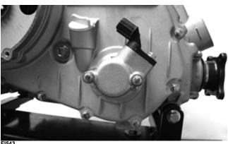
5. Remove the cap screws securing the magneto cover to the crankcase. Note the location of the two internal cap screws and the two longer cap screws.
