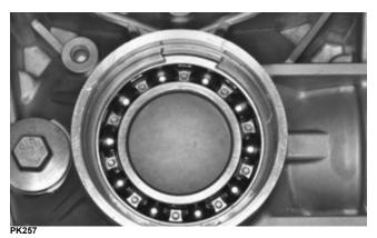
2. From the inside of the gear case cover, use a bearing driver adapter the same size as the outside race of the bearing and install. Lightly grease a new seal and install.
