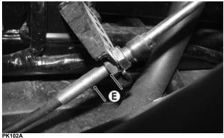
20. Remove the large and small diameter coolant outlet hoses from the cylinder head coolant fitting.
