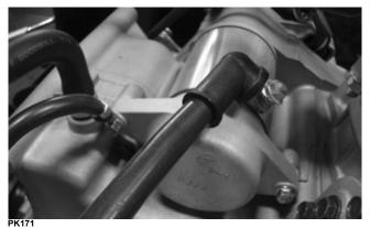
10. Place the throttle body into the intake boot and secure it with the clamp. Correctly route and secure the throttle cable using the routing clamps.
