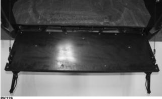
2. Secure each pivot panel using the two cap screws. Install each rear reflector panel using the two cap screws.
