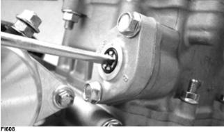
4. Bend the washer tabs and remove the two cap screws securing the sprocket to the camshaft.
