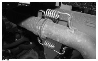
2. Slide the muffler assembly forward and clear of the holder pins. Account for the gasket.
