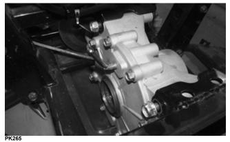
4. Using new patch lock cap screws, install and secure the rear brake caliper to the mount and tighten the screws to 19 ft-lb (25.8 N-m). Install the drive axles (see Drive Axles).
