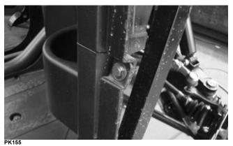
4. Install the left and right side panel assemblies using cap screws (A) and plastic rivets (B).
