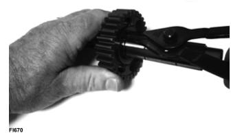
2. Install the high/low shift dog (6) on the countershaft and secure with snap-ring (7); then install the splined washer (8).
