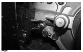
3. While holding the actuator firmly forward, tighten the front cap screw to hold the actuator in place; then install but do not tighten the two remaining cap screws.
