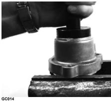
3. Grease the seal; then inspect and clean the sealing surface of the input shaft. Insert the input shaft into the bearing and secure with the snap ring.
