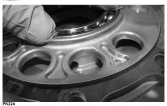
4. Verify the bearing flange is properly aligned with the different cover and fully seated. With the two dowel pins in place on the differential housing, place a new gasket into position.
