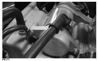
18. Wrap a shop towel around the fuel injector and rail. Remove the two cap screws securing the fuel rail to the cylinder head. Carefully remove the rail and injector. Account for the O-ring (A) on the injector then release the fuel line from the engine clamp (B). Secure the fuel line out of the way.
