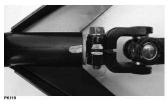
3. Align the match marks on the splined pinion shaft to the marks on the rack/pinion housing.
