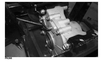
4. Pull the rear propeller shaft boots away from the input shaft and rear engine flange. Holding the propeller shaft in place, disengage the gear case from the propeller shaft moving it toward the rear. Account for the tension spring in the input shaft and boot spring clamps.
