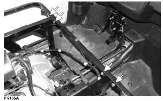
11. From each side of the vehicle, loosen the eight cap screws securing the outside of the seat frame to the top of the main frame.
