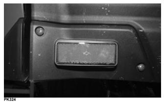
3. Remove the two cap screws securing both left and right pivot panels to the tailgate. Unlatch the tailgate from the cargo bed; then with the aid of an assistant, tilt the tailgate down and lift up to remove.
