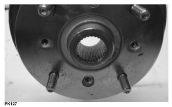
6. Install the hub assembly onto the splines of the shaft.
