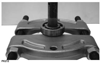
4. Inspect the pinion gear needle bearing. Using a suitable bearing puller, remove the needle bearing.
