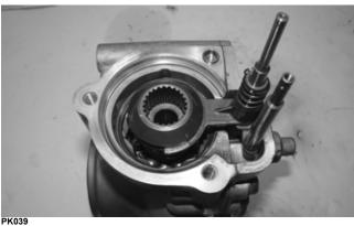
4. Remove the snap ring securing the input shaft; then slide it out of the housing.
