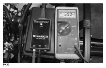
■NOTE: If the throttle body, ECM, TPS, or ISC are replaced, the EFI system must be synchronized. Use the following procedure:
