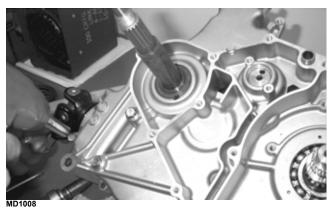
4. From the left side, install the remaining crankcase cap screws; then tighten only until snug.
