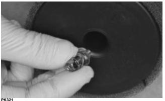
4. Slide out the air filter screen, then separate the inner and outer air filter elements to thoroughly clean.
