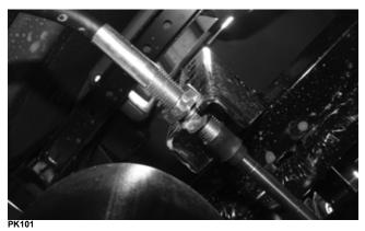
4. From under the seat, remove the E-clip (A) securing the cable end to the shift arm stud. Account for the washer (B) and bushing (C).
