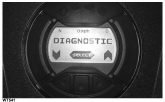
3. Press the center button (SELECT) to enter diagnostic mode; cycle the display by pressing either the left or right button to step to the desired function.
