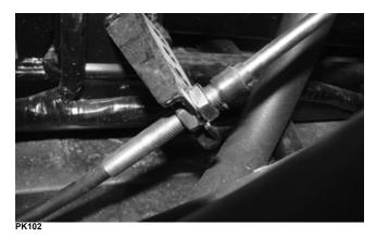
■NOTE: If the cable is being replaced, connect the new cable to the end of the existing cable and pull the new cable into place.
