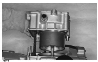
4. Loosely install the two nuts securing the cylinder to the right-side crankcase half.
