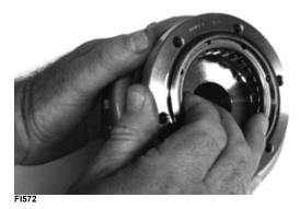
REPLACING STARTER CLUTCH ASSEMBLY
