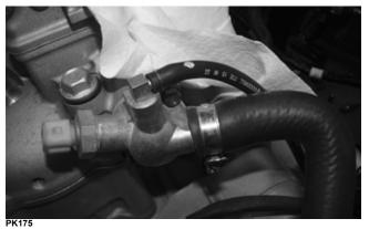
21. Remove both large and small diameter coolant return hoses from the water pump.
