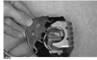
6. Remove the caliper holder from the caliper.
