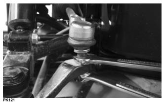
3. Remove the cap screws securing the steering rack assembly to the frame and remove from the left side.
