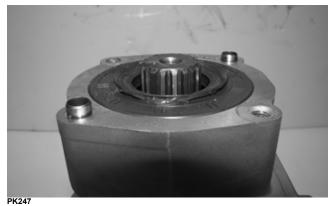
4. Place the gear case on its side; then remove the cap screws securing the housing cover to the housing. If necessary, use the pry point to aid in removal of the cover. Account for the cover side shim.
