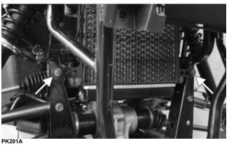
6. Lower the radiator through the front bumper. Account for two upper and two lower rubber mounting grommets.
