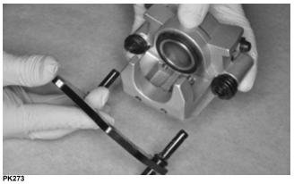
7. Cover the piston end of the housing with a shop towel; then keeping fingers clear of piston travel. Apply compressed air to the fluid port to blow the piston free of the housing. Account for the dust and piston seals.
