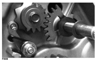
6. Install starter idler gears (1) and (2).
