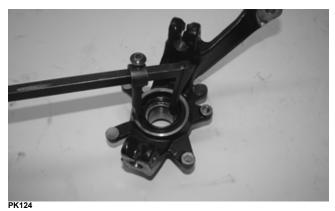
9. Remove the snap ring securing the bearing in the knuckle; then press the bearing out of the knuckle.
