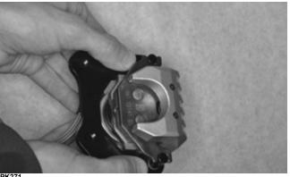
6. Secure the brake pads to the caliper with the brake pad pins. Apply blue Loctite to the threads of the pins; then tighten to 13 ft-lb (17.7 N-m).
