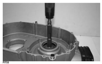
13. Remove the two Phillips head screws securing the bearing retainers to the inner clutch cover housing. Remove the retainers. Using an appropriately sized bearing driver set against the inner race of the bearing, press the bearing out of the clutch cover. Note the orientation of the bearing for assembly purposes.
