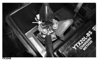
5. Engage the starter switch and observe the multimeter. The meter must show battery voltage.
