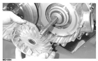
7. Remove the nut holding the driven pulley assembly; then remove the driven pulley assembly.
