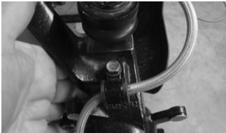
4. Secure the lower eyelet of the shock absorber to the lower A-arm. Tighten nut to 32.5 ft-lb (44.1 N-m).
