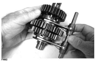
6. Remove the crank balancer driven gear (G) and account for a key; then remove the crankshaft balancer shaft.
