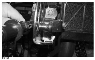
3. With the bushing (C) in place on the shift lever shaft, install the shaft cable. Secure it with a washer (B) and a new E-clip (A).
