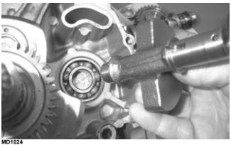
Install the key in the crank balancer shaft; then install the gear and aligning the timing marks, slide the gear into place.
