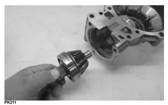
3. Place the pinion gear in a bearing puller or press blocks; then remove the pinion bearing using a press. Account for a collar and a bearing.
