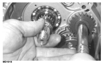
15. Remove oil pump drive gear. Account for the pin.
