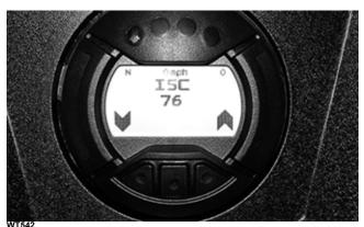
Display: ISC position DTC: P0508, P0509 Usage: Verify correct ISC position.
