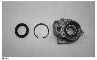
6. From the opposite side of the housing, use an appropriate sized bearing driver to press the bearing out of the housing.
