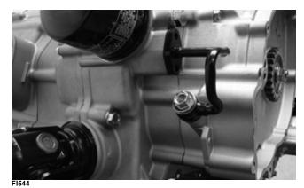
4. Remove the water pump drive gear; then remove the speed sensor housing assembly. Account for two alignment pins, a gasket, and two seal washers.
