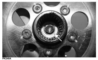
2. Remove the four cap screws securing the rear caliper mount to the gear case. Record the locations of the two different-length cap screws, which require patch-lock (A). Account for four crush washers.
