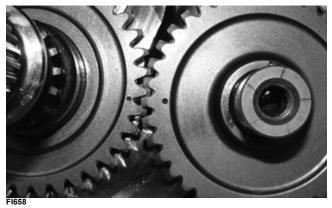
6. Align the shift cam fork slots with the shift fork shaft locating boss and with a washer on each end, install in the crankcase.
