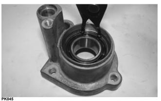
2. Install the input shaft seal, making sure it is fully seated in the housing.
