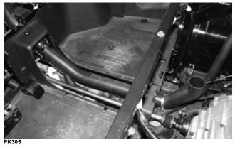
3. From the rear, remove the two cap screws securing the actuator to the differential and bracket.
