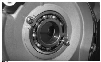
4. Lubricate the inner race of the centrifugal clutch housing bearing with engine oil; then using a bearing driver and ball peen hammer, drive the clutch housing into the bearing until it fully seats.
