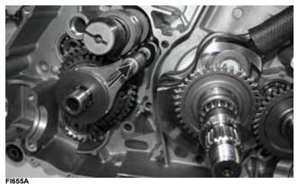
9. Install the input driveshaft.
