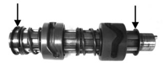
5. Remove the countershaft assembly (E) along with the shift fork assembly.
