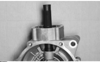
5. Using soft jaws, secure the gear case into a vise. Using a propane torch, heat the gear case to approximately 200° F (93° C); then carefully install the pinion gear assembly into the case. Install the lock collar to secure the pinion into the case. Using the Pinion Gear Lock Collar Socket, tighten to 125 ft-lb (169.5 N-m).
