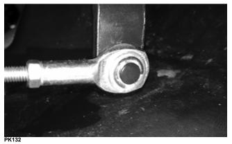
3. From under the front body panel, measure the installed length of the threads; then loosen the cable adjuster nuts. Slide the cable out of the bracket.
