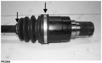
2. Using a pick or small flat blade screw driver, remove the circlip stop ring (A) from the CV housing. Remove the housing.
