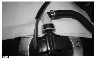
2. Connect the fuel line to the fuel pump; then verify the connector is fully seated to the fuel pump juncture. Connect the fuel pump harness connector to the main wiring harness.
