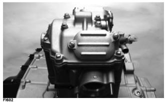
29. Install the spark plug and tighten securely; then install the timing inspection plug.
