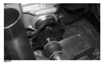
23. Remove the cap screws securing the front engine cradle to the frame; then remove the lock-nuts securing the rear engine cradle to the frame. Discard the lock nuts.
