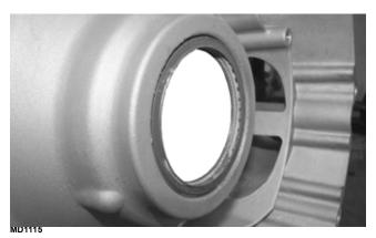
3. Place a new bearing into position with the sealed side of the bearing facing down; then using an appropriately sized bearing driver, press the bearing via the outer race into the inner clutch cover. Apply blue Loctite #243 to the threads of the two Phillips head screws and secure the two retainers.
