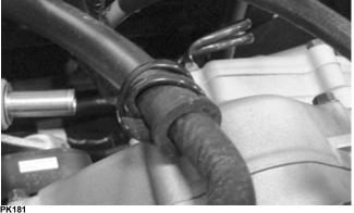
9. Place the starter cable onto the starter motor and secure it with the nut. Secure the engine ground cable to the engine using the front starter motor mount cap screw. Tighten securely.
