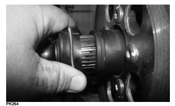
5. Tilt the gear case on its right side; then move it forward through the frame. Remove the gear case from the right side of the frame.
