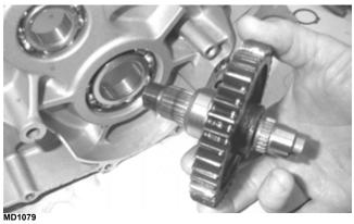
2. Install and tighten the output shaft flange nut to 59 ft-lb (80.2 N-m). Using a punch, peen the nut.
