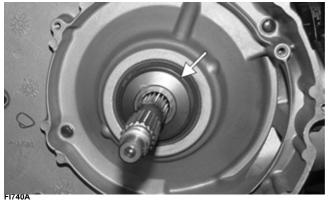
6. Install two alignment pins and place the clutch cover gasket into position. Install the inner clutch cover.
