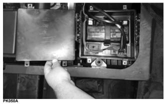
2. Remove the battery by disconnecting the negative cable first then the positive cable. Move the starter relay and cables up out of the way. Remove the four cap screws securing the battery box to the frame.
