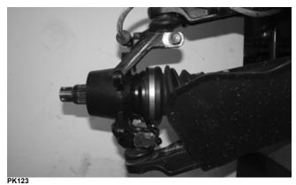
4. Install the tie rod end onto the knuckle; then install the washer and secure with the nut (coated with red Loctite #271). Tighten to 30 ft-lb (40.8 N-m); then install a new cotter pin and spread the pin.
