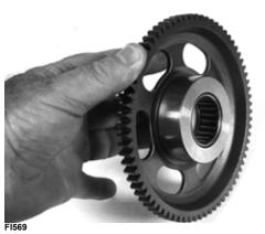
3. Inspect the one-way bearing for chipped surfaces, missing rollers, or discoloration. If any of the above conditions exist, replace the starter clutch assembly.
