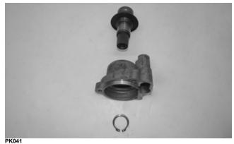
5. To gain access to the housing bearing, remove the seal and snap ring from the input shaft housing.
