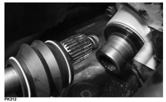
13. Protect the painted surface of the frame; then tilt the differential assembly on its left side. Remove through the front of the frame.
