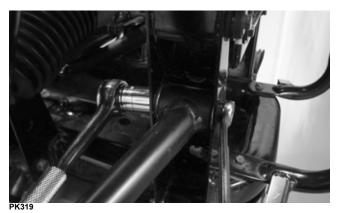
3. Route the brake hose along the upper A-arm. Secure with hose and clamps.
