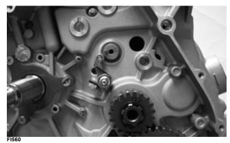
13. Remove the snap ring securing the output drive gear to the output shaft and remove the gear noting that the hub flange is directed toward the crankcase.
