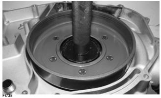
5. With a new O-ring installed into the spacer, place the spacer over the centrifugal clutch housing shaft and fully seat it into the inner clutch cover seal.
