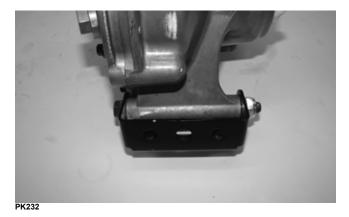
2. Grease the input shaft and front propeller shaft splines. Insert the tension spring (A) into the propeller shaft. Place the differential assembly into position in the frame engaging the front propeller shaft; then install the top mounting cap screw and new lock nut. Do not tighten at this time. Slide the propeller shaft boot with the two spring clamps over the input shaft coupling.
