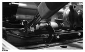
5. Align the match marks made on the front and rear drive flange assemblies. Install the eight cap screws and tighten to 20 ft-lb (27.2 N-m).
