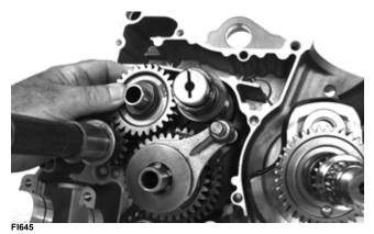
11. Install the secondary output driveshaft assembly into the crankcase half making sure the front and rear bearing alignment pins are seated in the recesses; then install the center carrier bearing alignment Cring.
