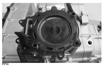
7. Install the four cylinder head cap screws with washers. Tighten only until snug. Note that the two cap screws on the right side of the cylinder head nearest the cam sprocket are longer than the two cap screws on the left (spark plug) side. Tighten only until snug.
