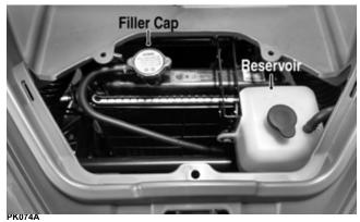
2. Remove the radiator cap; then drain the coolant into a suitable container by removing the drain plug found on the water pump. Account for the washer. Disconnect the cooling fan wire connector from the main harness.
