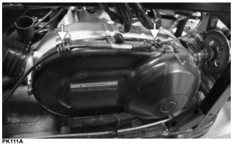
17. Remove the starter cable from the starter motor; then remove the engine ground cable from the front starter motor mount.
