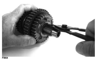
5. Install the reverse dog on the shaft; then place the shift forks and shift shaft into position.
