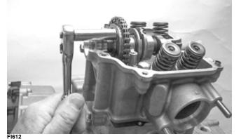
5. Using an awl, rotate the C-ring in its groove until it is out of the cylinder head; then remove the C-ring.
