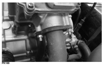
16. Remove the spark plug cap from the spark plug. Disconnect the coolant temperature sensor (A), TPS (B), ISC (C), TMAP (D), and fuel injector (E) connectors. Secure the harness out of the way. Loosen the clamp securing the throttle body to the intake boot. Note the throttle cable routing and release the throttle cable from the clamps attached to the top of the CVT housing; then secure the throttle body out of the way.
