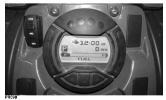
Move the shift lever all the way forward. The letter L should illuminate on the LCD gauge.
