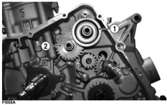
7. Install the starter clutch gear onto the crankshaft; then install the rotor/flywheel key in the crankshaft.
