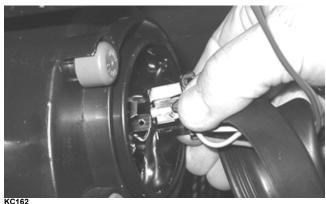
2. Press in and release the spring retainer and pull rearward clear of the bulb assembly.
