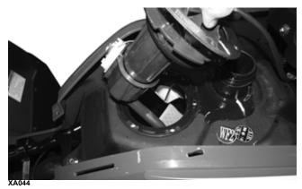
3. Rotate the fuel pump until the match marks align; then install the mounting screws and tighten securely using a crisscross pattern.
