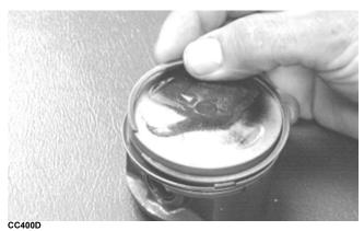
2. Remove each ring by working it toward the top of the piston while rotating it out of the groove.
