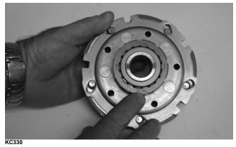
2. Place the clutch housing onto the clutch shoe/one-way clutch.
