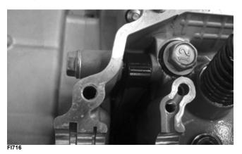
12. With the alignment pin installed in the camshaft and the cam lobes directed down (toward the piston), place the camshaft in position and verify that the timing mark on the magneto is visible through the inspection plug and that the timing marks on the camshaft sprocket are parallel with the cylinder head cover mating surface.
