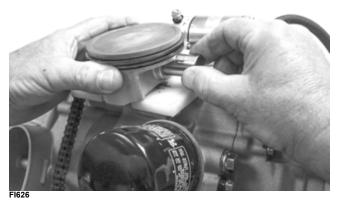
2. Place the two alignment pins into position. Place a new cylinder gasket into position; then place a piston holder (or suitable substitute) beneath the piston skirt and square the piston in respect to the crankcase.
