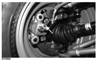
2. Place an absorbent towel around the connection to absorb brake fluid. Remove the banjo-fitting bolt from the master cylinder. Account for two crush washers and a banjo-fitting bolt.
