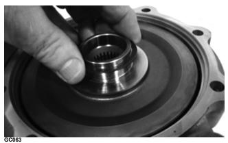
4. Place the differential with the open side down; then lift the housing off the spider assembly. Account for shim(s) and mark as right-side.
