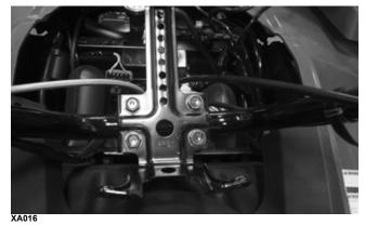
4. Remove the cap screws securing the upper steering post to the frame. Account for the housing cap, outer housing, and inner housing.
