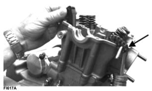
7. Remove the cam chain tensioner pivot bolt and remove the chain tensioner; then remove the two nuts securing the cylinder head to the cylinder.
