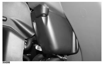
6. Remove the screws securing the front body to the front body supports.
