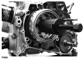
9. Remove the flywheel key from the crankshaft; then remove the starter clutch gear.
