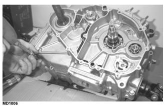
2. Using Crankcase Separator/Crankshaft Remover and tapping lightly with a rubber mallet, separate the crankcase halves. Account for two alignment pins.
