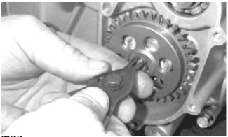
■NOTE: Always use a new snap ring when installing the oil pump driven gear.
