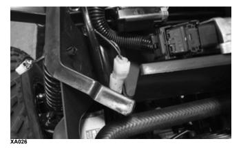
■NOTE: To determine if the fan motor is good, connect the blue wire from the fan connector to the positive side of a 12-volt DC power supply; then connect the black wire from the fan connector to the negative side. The fan should operate.
