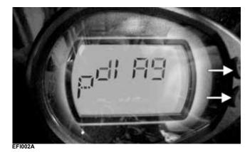
■NOTE: The display on the gauge will display in SAE (speedometer in MPH mode) or Metric (speedometer in km/h mode), For example to read temperature in degrees Celsius, select km/h mode on the gauge or to read Fahrenheit, select MPH mode.
