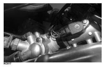
■NOTE: Prior to testing the TPS, inspect the three-wire plug connector on the main harness and the three-pin plug on the TPS for contamination, broken pins, and/or corrosion.
