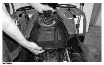
7. Remove the cap screw (A) securing the gas tank to the frame; then disconnect the fuel hose (B) and fuel pump connector (C). Remove the gas tank to the rear. Account for the heat shield.
