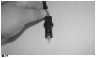
2. Push a new bulb into the socket; then place the socket into the light housing and turn clockwise to secure.
