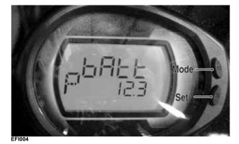
■NOTE: The gauge can be utilized dynamically (engine running/vehicle moving) or statically (engine/vehicle stopped).
