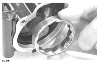
6. Using the Pinion Gear/Shaft Removal Tool and a hammer, remove the pinion gear from the gear case housing.
