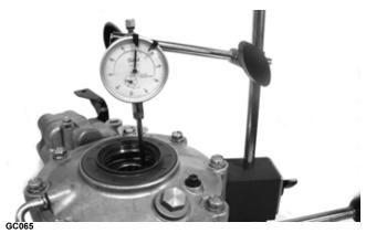
2. Zero the dial indicator; then push the ring gear toward the dial indicator and release. End-play should be 0.004-0.008 in. (0.102-0.203 mm).
