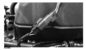
5. Connect a multimeter to the power supply leads with the red tester lead to the red wire and the black tester lead to the black wire; then turn the ignition switch to the ON position. The meter should read battery voltage. If battery voltage is indicated and the fuel pump does not run, replace the pump assembly. If no battery voltage is indicated, check the fuel relay, 10-amp fuel fuse, main relay, main fuse, ECM and the vehicle tilt sensor.
