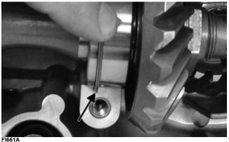
2. Remove the reverse idler assembly (B). Account for and note the location of the inner bushing (1), idler shaft (2), and outer washer (3).
