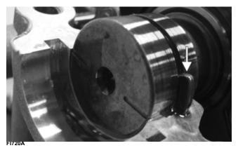
6. Noting the timing marks for installing purposes, drop the sprocket off the camshaft. While holding the cam chain, slide the sprocket and camshaft out of the cylinder head. Account for an alignment pin.
