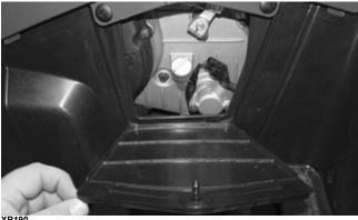
4. Remove the drain plug from the bottom of the engine and drain the oil into a drain pan.
