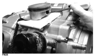
14. Using Piston Pin Puller, remove the piston pin.
