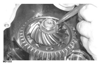
3. Apply a liberal amount of oil to the crankshaft bearing. Using a propane torch, heat the bearing until the oil begins to smoke; then slide the crankshaft assembly into place.
