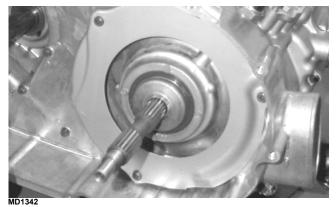
10. Place the driven pulley assembly into position and secure with the nut (threads coated with red Loctite #271). Tighten to 147 ft-lb (199.3 N-m).
