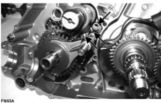
4. Remove the gear shift shaft (F) noting the inner and outer washers.
