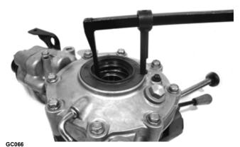
2. Using a press, remove the bearing.
