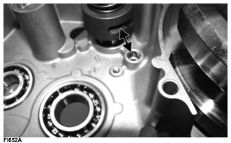
7. Place the shift forks into position on the assembled countershaft and install into the crankcase as an assembly.
