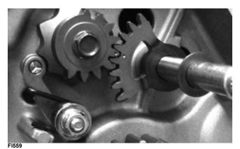
6. Install starter idler gears (1) and (2).
