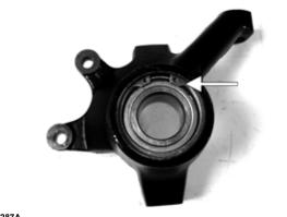
2. Install the knuckle to the upper and lower ball joints and secure with the two cap screws. Tighten to 35 ft-lb (47.6 N-m).
