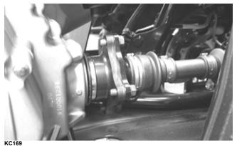
3. Remove the two cap screws and lock nuts securing the rear gear case to the frame; then remove the gear case through the left side.
