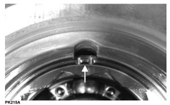
5. Install the pinion housing.
