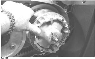
3. With two drops of red Loctite #271 on the threads and with the splines of the clutch shaft protruding through the movable drive face, install the nut and tighten to 147 ft-lb (199.3 N-m)
