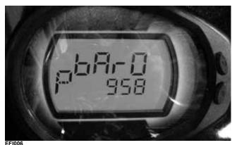
Display: MAP in millibars (1013 millibar = 29.92 in. mercury).
