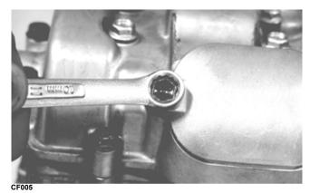
2. Rotate the crankshaft to the TDC position on the compression stroke.
