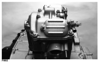
29. Install the spark plug and tighten securely; then install the timing inspection plug.
