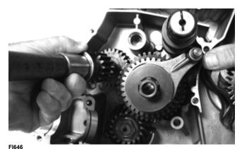
10. Install the spacer (1), shaft (2), reverse idler gear, and washer (3).
