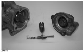
5. Install the shift fork assembly making sure the fork leg is facing upward. Apply a small amount of oil to the gasket; then install the gasket dowel pin.
