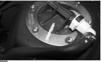
5. Disconnect the gas line connector from the fuel pump outlet.
