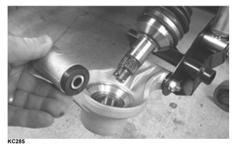
7. Place a drain pan under the ATV to contain any oil leakage; then pull out sharply on the axle to dislodge the splines from the gear case. Remove the axle.
