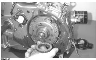
12. Remove the left-hand threaded nut holding the centrifugal clutch assembly.
