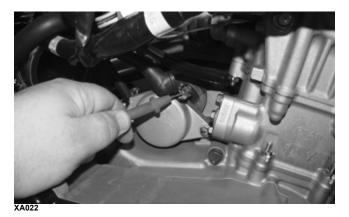
■NOTE: If the meter showed correct voltage but the starter did not operate or operated slowly, the starter motor is defective.
