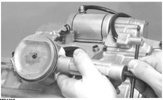
■NOTE: Support the connecting rod with rubber bands to avoid damaging the rod or install a connecting rod holder.
