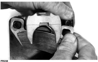
6. Remove the caliper holder from the caliper and discard the O-ring.
