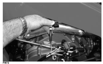
3. Using a multimeter, connect the black tester lead to the black socket (GND) on the analyzer and the red tester lead to the white socket (VAR); then select the DC Voltage position. With the vehicle off, the gauge should read 0.66-0.70 and at Wide-Open Throttle it should read up to approximately 3.88.
