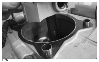
3. Lubricate the inside wall of the cylinder; then using a ring compressor or the fingers, compress the rings and slide the cylinder over the piston. Route the cam chain up through the cylinder cam chain housing; then remove the piston holder and seat the cylinder firmly on the crankcase.
