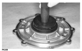
■NOTE: Prior to installing the seal, apply High Performance #2 Molybdenum Disulfide Grease to the seal outside diameter.
