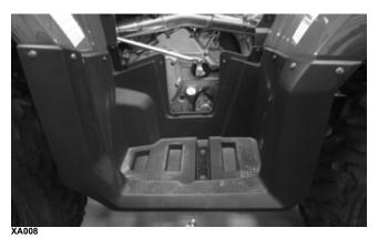
8. Remove the front body panel/fender panel.
