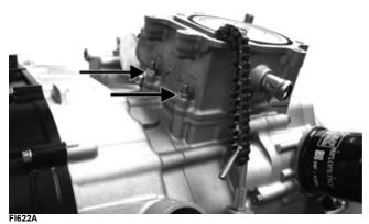
12. Lift the cylinder off the crankcase taking care not to allow the piston to drop against the crankcase. Account for the gasket and two alignment pins.
