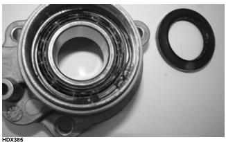
2. Install the input shaft seal making sure it is flush with the edge of the housing.
