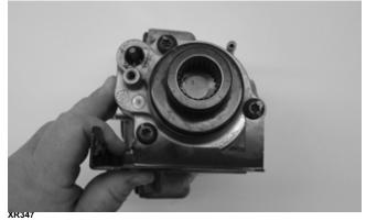
5. Lubricate the input shaft splines with High-Performance #2 Molybdenum Disulfide Grease.
