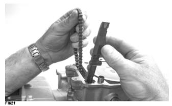
6. Place a new gasket into position on the cylinder. Place the alignment pins into position; then place the head assembly into position on the cylinder making sure the cam chain is routed through the chain cavity.
