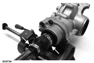
7. Using a new O-ring lubricated with grease.
