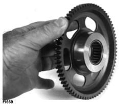
3. Inspect the one-way bearing for chipped surfaces, missing rollers, or discoloration. If any of the above conditions exist, replace the starter clutch assembly.
