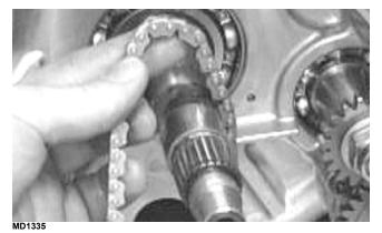
14. Remove the oil pump drive gear cap screw.
