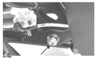
2. Slide the auxiliary brake pedal part way off the pivot stud but do not remove; then remove the cap screws from the V-belt housing and remove the cover. Account for two alignment pins and a gasket.
