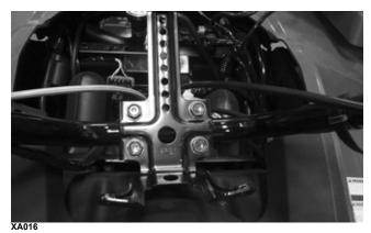
5. Install the steering post cover; then install the left-side fender well and front access panel.
