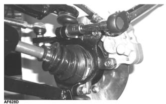
5. Install the hub to the axle; then tighten the nut to specification and secure with cotter pin. Install the brake caliper.
