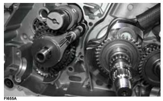
9. Install the input driveshaft.
