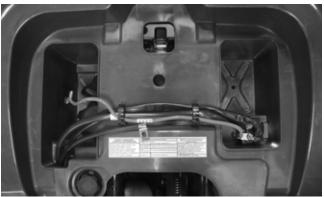
4. Using a small screwdriver, remove the light connectors from the frame; then disconnect both connectors and remove the rear body panel/fender.
