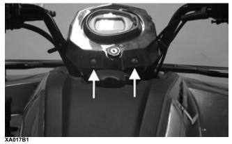
3. Remove the cap screws (A) securing the rear of the front body to frame; then remove the two reinstallable rivets (B) securing the gas tank cover to the body.
