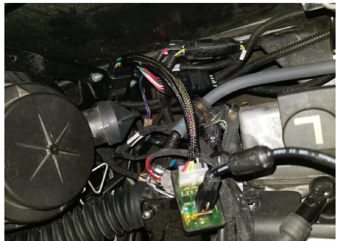
Fig. 8 Jumper harness installed in vehicle
