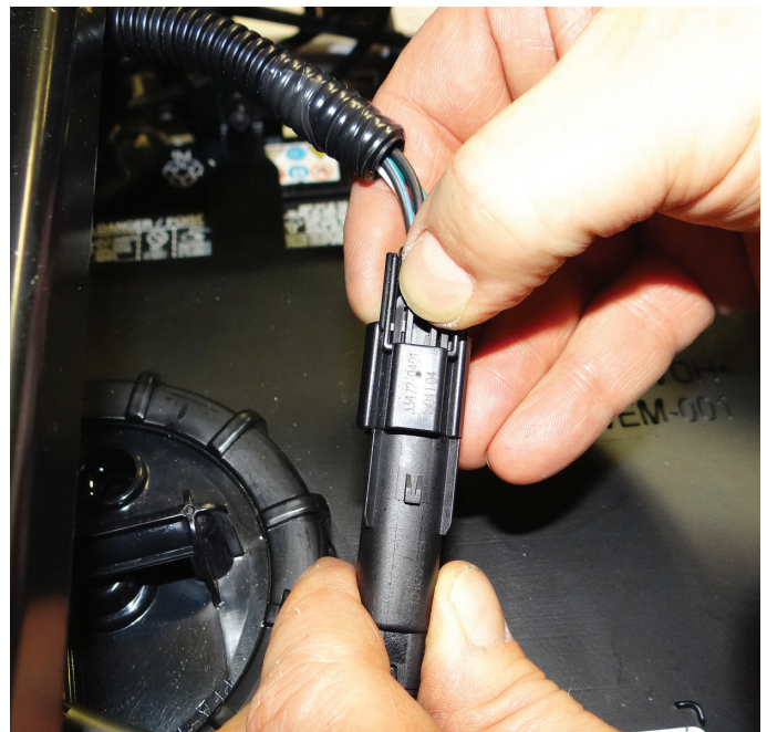
Fig. 2 Fuel Pump Wire
