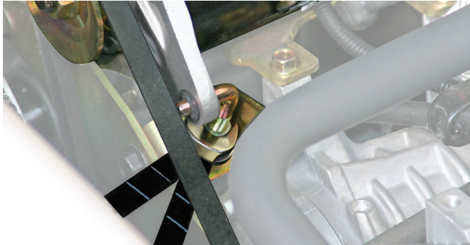
Fig. 11 Adjusting the Belt Tension
