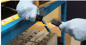
Figure 1: Disconnect AC power.
