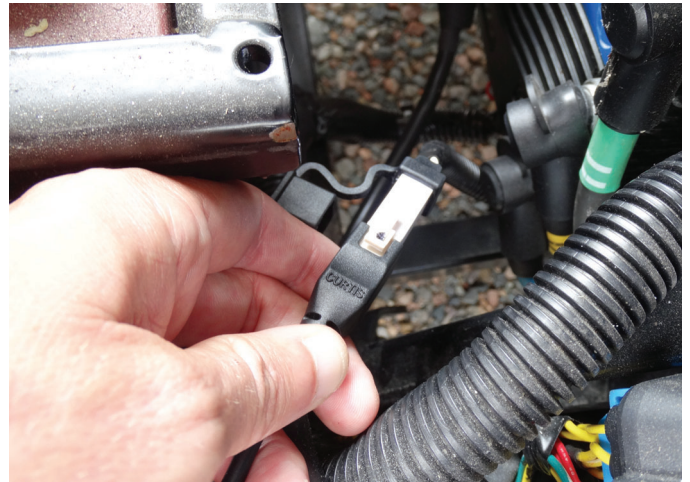
Fig. 4 Curtis Programmer Port Installation
