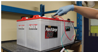
Figure 2: Remove positive lead from positive terminal on the battery pack.
