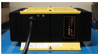
Figure 4: Charger LED indicator self-test.
