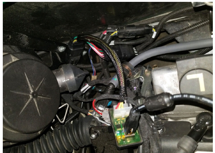
Fig. 8 Jumper harness installed in vehicle
