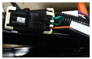
Fig. 5 Motor Brake Jumper
