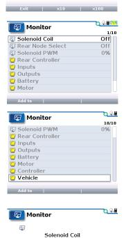
The "Monitor" menu selection shows controller functions, inputs, and outputs.
