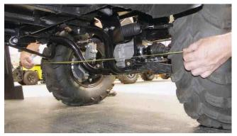
Fig. 15 Wheel Alignment Rear of Front Tires
