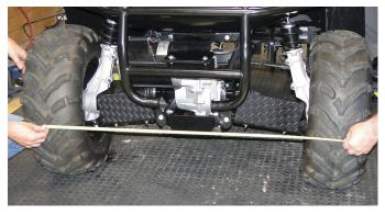
Fig. 14 Wheel Alignment Front of Front Tires
