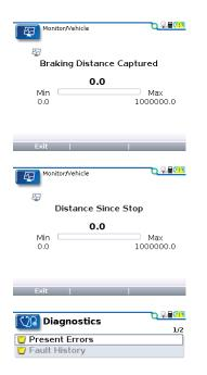
"Braking Distance Captured" indicates the distance traveled by the vehicle starting with the vehicle braking (initiated by throttle reversal, brake pot, VCL Brake, or interlock braking) and ending when the motor RPM = 0. Units are measured in feet.
