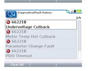
"Fault History" shows faults encountered by the controller in the past. Specifics of when the fault occurred in run time hours can be viewed by selecting each fault directly.
