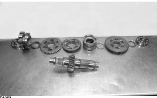
4. Inspect the dogs for nicks, cracks, chips, or signs of wear. If any are present, the dog must be replaced.
