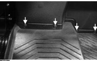
Remove the two cap screws located near the front tires securing the splash panel to the floor on each side.
