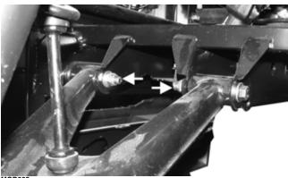
3. Route the brake hose along the upper A-arm. Secure with hose anchors and the clamp.
