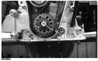
9. Install a new timing belt keeping the timing marks aligned; then push tensioner arm in the direction of the arrow until the gap between the tensioner and water pump housing is 5 mm (0.2 in.) and tighten the tensioner cap screw securely.
