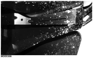
2. Remove the three shouldered cap screws from the top of the side cover and the two shouldered cap screws from the bottom of the side cover.
