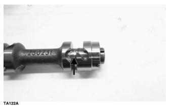
7. While holding pressure on the washer, rotate the cam counterclockwise to lock the cam onto the shift drum.
