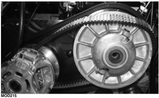
7. With the driven clutch still on the transaxle input shaft, place the Drive and Driven Clutch Holder Tool on the drive and driven clutch to hold the drive clutch in place; then with a Torx T-60 drive, remove the cap screw securing the drive clutch. Account for the washer.
