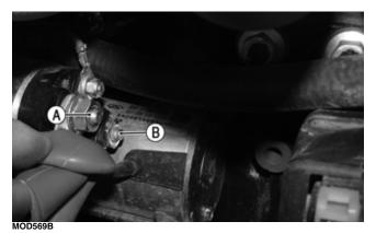
3. With the brake depressed, rotate the key switch to the starter position while observing the multimeter. The multimeter should drop to 0 volts, the starter should engage, and a "click" should be heard from the relay.
