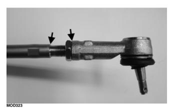
4. Using a wrench, loosen the lock nut (B) while holding the tie rod at the location indicated (C); then remove the tie rod with a wrench at the location indicated (C) while holding the tie rod shaft at the location indicated (A).
