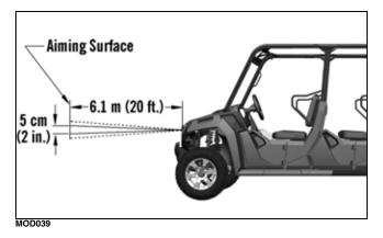
■NOTE: There should be an average operating load on the vehicle when adjusting the headlight aim.
