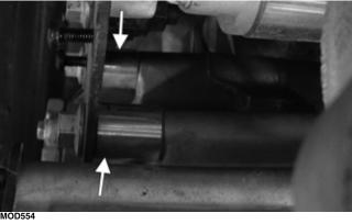
7. Remove the two cap screws securing the starter to the engine backplate; then use a suitable strap to support the starter; then remove the two cap screws securing the engine backplate to the front engine mount; then remove the four cap screws securing the engine backplate; then remove the engine backplate.
