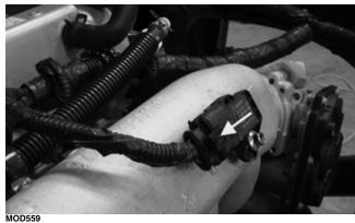
13. Install the coolant sensor connector to the coolant sensor; then connect the coil connectors to the coils; then install the engine oil pressure switch connector to the engine oil pressure switch that is located near the engine oil filter; then attach the engine ground located above the engine oil pressure switch.
