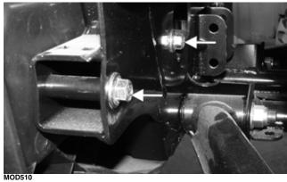
3. Install the two cap screws located below the front tow hooks.
