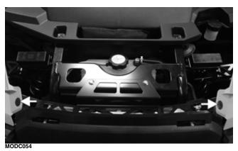
5. Pour the recommended coolant into the coolant reservoir; then bleed the system (see Bleeding Cooling System in this section).
