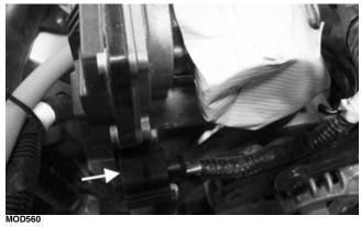
18. Gently remove the engine from the chassis, being careful of any electrical components, hoses, straps, and etc.
