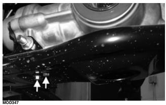
2. Remove the upper mount cap screw and lock nut for the front differential; then remove the four cap screws securing the upper differential mount; then remove the upper differential mount.
