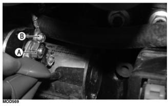
3. Remove the two cap screws securing the starter; then remove the starter. Account for the dowel pins.
