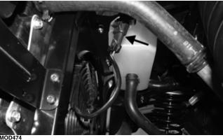
5. Lift the radiator assembly from the vehicle. Account for two upper and two lower rubber mounting grommets.
