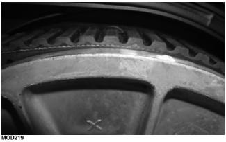
9. Install the clutch cover making sure the gasket is completely in the grove on the engine side. Install six clamps securing the clutch cover
