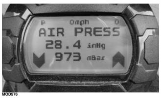
Display: Air pressure as measured by the Temperature Manifold Absolute Pressure (TMAP) sensor
