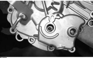
■NOTE: It will be necessary to tap the cover onto the case using a rubber mallet. Ensure the alignment pins are properly oriented.
