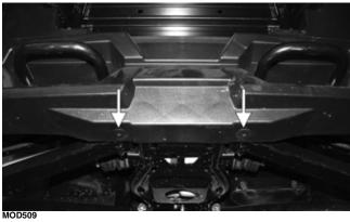
2. Remove the two cap screws behind each tow hook and then remove the tow hooks.
