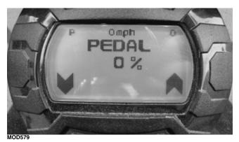
Display: Accelerator position sensor percentage as measured by the accelerator position sensor.
