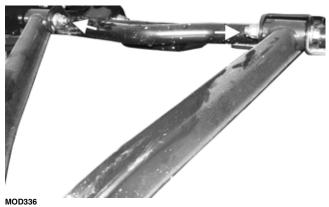
8. Remove the snap ring from the ball joint; then remove the ball joint from the A-arm.
