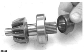
2. Place the pinion assembly in a bearing puller; then install the bearing using a press.
