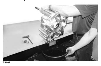
■NOTE: Tip the transaxle toward the drain to get any remaining fluid.
