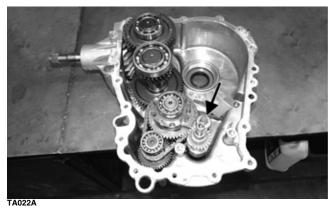
5. Using an assistant, lift and remove all remaining shafts simultaneously.
