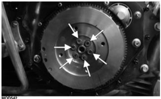
10. Install the crank position sensor into the crankshaft position sensor bracket and tighten to 8 ft-lb (10.9 N-m). Install the PTO stub shaft and tighten cap screws to 36.9 ft-lb (50 N-m). Install the flywheel cover and tighten cap screws securely.
