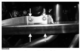
5. Located on the PTO side, install the two cap screws with blue Loctite #243 with the spacers between the engine and transaxle. Tighten to 75 ft-lb (102 N-m).
