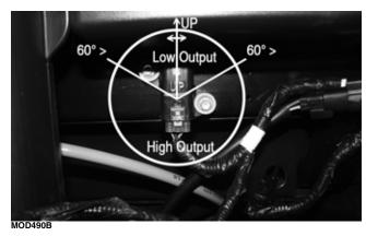
■NOTE: When replacing the sensor after testing, make sure the arrow marking is directed up.
