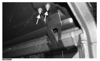
Remove the cap screws and lock nuts at the front of the roof. Account for the washers and the lock nuts. Remove the roof.
