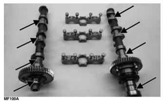
10. Inspect the camshaft lobes for flaking, galling, scoring, or bluing indicting heat build-up. If damaged or worn beyond limits, camshafts will have to be replaced.
