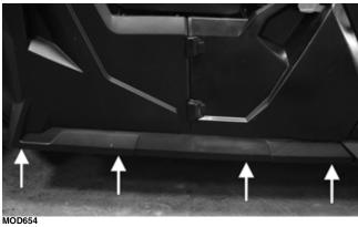
4. Remove the four cap screws securing the door hinge and remove the door hinge; then remove the remaining cap screws securing the side panel; then remove the side panel.
