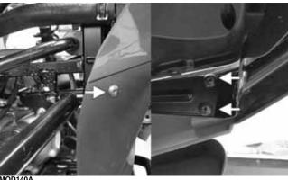
4. Remove the two T30 shouldered cap screws from the center of the front fascia; then remove the front fascia.
