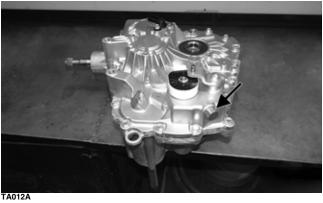
3. Remove and discard the lock nut securing the bell crank; then using two screwdrivers, pry the bell crank off the shift shaft.
