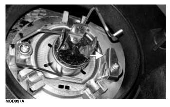
3. Install the rubber boot making sure it is sealed around the bulb and connect the wire harness.
