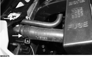
4. Remove the two cap screws and lock nuts securing the radiator bracket to the frame; then remove the radiator bracket from the vehicle; then disconnect the
