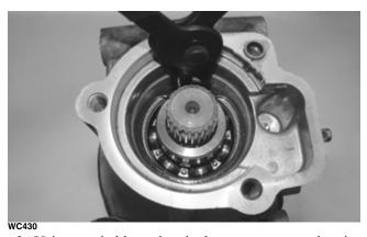
2. Using a suitable tool and a hammer, remove the pinion gear from the gear case housing.
