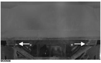
With the help of an assistant or an adequate lift, remove the cargo box from the vehicle. The cargo box tilt lever will need to be released.
