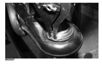
2. Install the A-arm assemblies into the frame mounts and secure with the cap screws. Only finger-tighten at this time.
