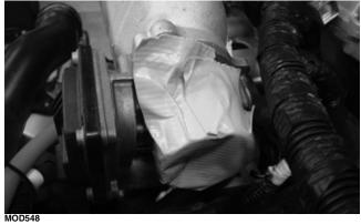
11. Remove the two cap screws and nuts securing the exhaust to the exhaust manifold; then gently pull the exhaust from the exhaust manifold.
