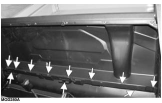
Remove the two cap screws on each seat belt guide; then remove seat belt guides; then disconnect the seat belt electrical connector.
