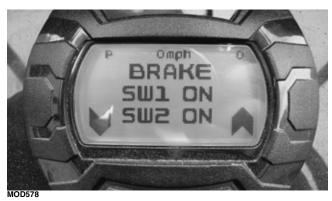
Display: Brake switch signal from switch 1 (front) and switch 2 (rear).
