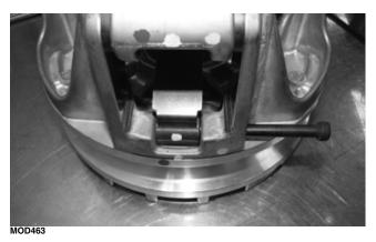
■NOTE: Grasp the movable sheave and lift it upward; then release it. It must move freely and not bind at any point.
