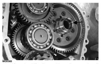
4. Lift on the shift rail assembly to disengage the rail assembly from the case and rotate the rail away from the shift drum; then remove the shift drum assembly.
