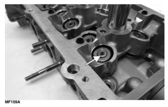
■NOTE: Collets can be held in position during assembly by applying a small amount of grease to the inner surface of the collets.
