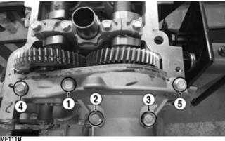
18. Install the camshaft drive belt and covers making certain that the camshafts are correctly timed to the crankshaft (see REMOVING AND INSTALLING CAMSHAFT DRIVE BELT in this section).
