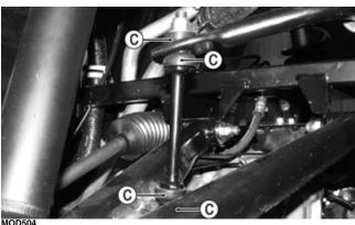
3. Remove the two cap screws per side securing the sway bar to the frame; then remove sway bar from frame.
