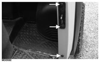
4. Install the four cap screws in the inner fender.
