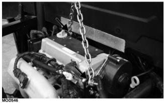
7. Remove the two cap screws securing the engine to the transaxle. Account for the spacers and washers between the engine and transaxle.
