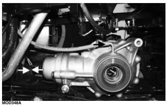
2. Install the lower differential mounting cap screws. Do not tighten at this time. Reconnect the front drive actuator connector above the front drive actuator (A) to the main harness and secure with nylon ties.
