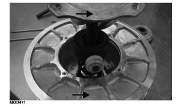
6. Using a suitable compressor, put a light amount of pressure compressing the driven clutch; then install the four cap screws securing the cam to the driven clutch. In a crisscross pattern, tighten to 47 in-lb (5.3 N-m).
