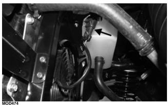
2. Remove the four cap screws securing the fan to the radiator fan bracket; then remove the fan from the radiator.
