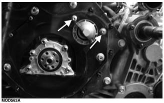
4. Install the four cap screws at the front of the engine below the engine oil filter. Tighten to 55 ft-lb (74.8 N-m).
