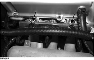
9. Install the air inlet tube to the throttle body and tighten the clamp securely; then insert the throttle control connector (6) into the receptacle in the throttle body and seat securely.
