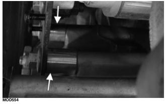
8. Remove the two cap screws securing the starter to the engine backplate; then remove the starter; then remove the two cap screws securing the driver-side backplate to the front mount; then remove the four cap screws for the engine backplate and remove the engine backplate.
