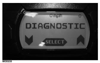
3. Press the center button (SELECT) to enter diagnostic mode; cycle the display by pressing either the left or right button to step to the desired function.
