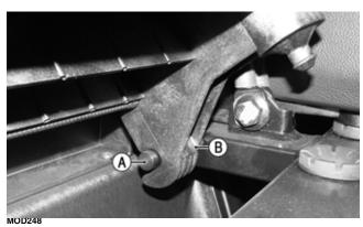
2. Install the seat bottom by hooking both of the "C" channels of the seat bottom into the mounting pegs (A).
