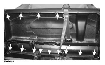
2. Reinstall the cap screw on each of the outer portions of the behind-the-seat storage box panel.
