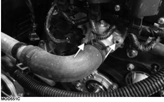
3. Install the coolant hose to the thermostat housing; then pour the recommended coolant into the coolant reservoir; then bleed the system (see Bleeding Cooling System in this section).
