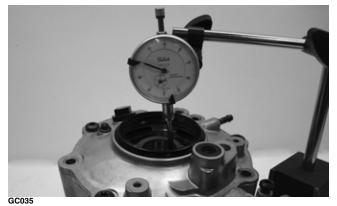
Zero the dial indicator; then push the ring gear toward the dial indicator and release. End-play should be 0.004-0.008 in. 3. To increase end-play, decrease the shim thickness. To decrease end-play, increase the shim thickness.
