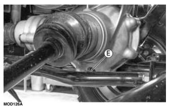
Located above the front drive actuator (A). Disconnect the front drive actuator connector from the main harness.
