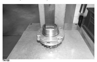
7. Install the large outer snap ring with the shim.
