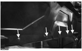
5. Remove the five cap screws near the cup holders; then remove the behind-the-seat close off panel.
