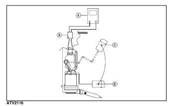
■NOTE: If readings are erratic, clean the resistor wiper and resistor with clean alcohol and retest. If still not correct, replace the fuel pump assembly.
