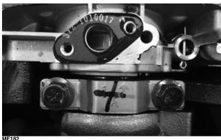
5. Remove the cap screws securing the oil pump assembly to the engine block and remove the oil pump assembly. Account for two rubber weatherstrip seals and a case gasket.
