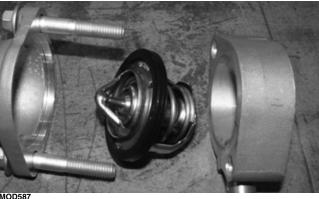
2. Install the two cap screws securing the thermostat housing and tighten to 15 ft-lb (20 N-m).
