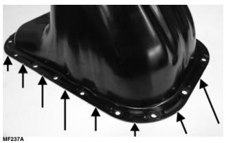
4. Apply a thin line of high temperature silicone sealant around the sealing surface of the oil pan as illustrated; then place the oil pan into position on the engine block and secure with the cap screws and tighten evenly to specifications.
