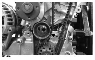
■NOTE: It is not advisable to reuse the timing belt once removed from the pulleys due to set wear patterns not realigning. The belt may be reused if:
