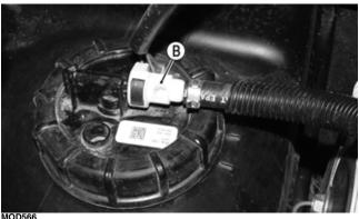
4. Mark the fuel pump mounting and gas tank for installing purposes; then using a suitable tool, remove the fuel tank nut securing the fuel pump to the gas tank and remove the fuel pump.
