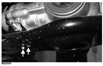
9. Install the upper differential mounting bracket and cap screws. Tighten to 16 ft-lb (21.8 N-m).
