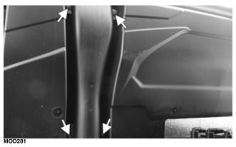
3. Remove the 11 cap screws securing the passenger seat backrest hinge; then remove the passenger seat backrest hinge.
