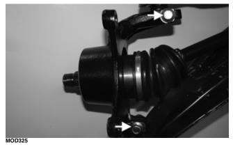
7. Secure the lower shock eyelets with cap screws and lock nuts. Tighten to 45 ft-lb (61.2 N-m).
