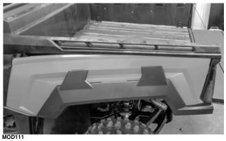
9. Once the outer side panel is in place, install the screws securing the cargo box fender and outer side panel.
