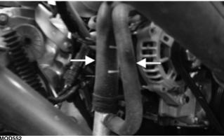
■NOTE: Coolant will come out when removing the coolant hoses. It is recommended to have a drain pan or suitable absorbant material near when removing coolant hoses.
