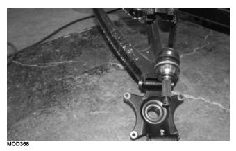
■NOTE: The axle shaft must be pushed into the inner CV joint straight.
