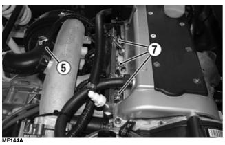
11. Install the fuel hose connector onto the fuel rail; then install the P-clamp holding the fuel line to the intake manifold; then install the coil pack onto the cylinder head and secure with the two cap screws and lock nut. Tighten securely.
