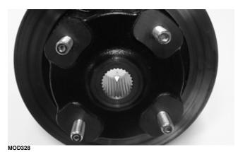
5. Install the hub assembly onto the splines of the shaft.
