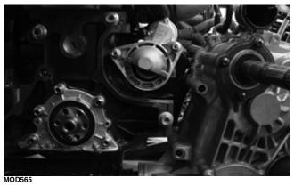
8. Uncouple the driveshaft from the transaxle by gently sliding the front differential with the driveshaft toward the front of the vehicle. Account for the O-rings and boot for the driveshaft-to-transaxle coupler.
