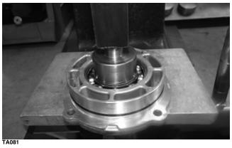
6. Using an appropriate bearing installer, install a new bearing into the housing.
