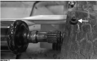
6. Gently pull the front driveshaft away from the front differential and account for the rubber bumper; then remove the front driveshaft from the vehicle.
