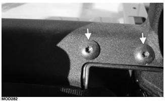
5. Remove the cap screw on each of the outer portions of the behind-the-seat storage box panel.
