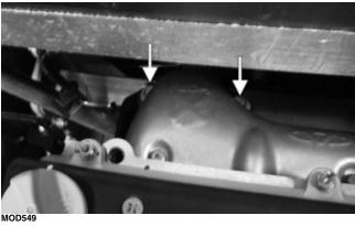
Disconnect the fuel hose connector from the fuel rail; then remove the P-clamp holding the fuel line to the intake manifold.
