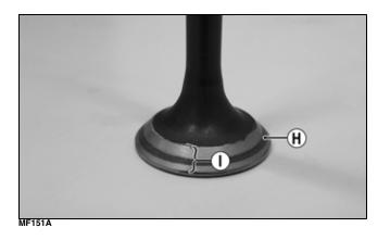
Wash all parts in cleaning solvent to remove lapping compound and dry with compressed air.
