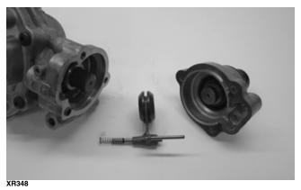
3. Remove the snap rings from the input shaft; then remove the input shaft from the pinion housing.
