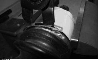
2. Use a suitable form of protection on the outside surface of the CV joint, such as a strip of rubber or duct tape; then place the CV joint housing into a vise.
