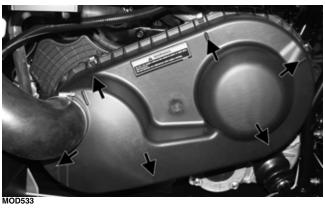
8. Connect clutch air inlet to snorkel portion; then install the clamp that holds the snorkel portion to the air inlet.
