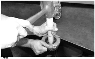
4. Remove the large outer snap ring and account for the shim.
