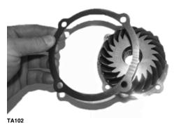
8. If backlash measurement is more than specified, remove the existing shim and install a thinner shim.
