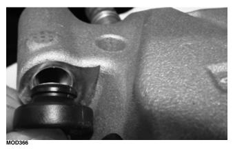
2. Apply high temperature silicone grease to the caliper mounting bracket rods; then install the caliper mounting bracket into the caliper.
