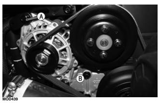
4. Remove the adjuster cap screw and pivot bolt and remove the alternator.
