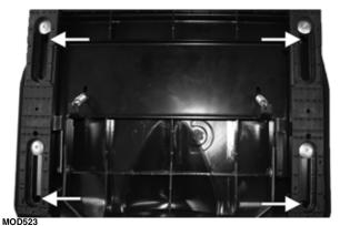
2. Position the seat backrest to the seat assembly; then install the four cap screws securing the seat backrest to the seat assembly. Torque to 2 ft-lb (2.7 N-m).
