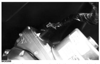
2. Align the steering rack with the marks with the wheels straight ahead.
