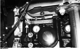
14. Install the driver-side coolant hose to the engine; then install the coolant hose above the starter; then install the coolant hose near the engine intake.
