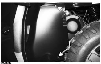
3. Loosen the clamp that holds the snorkel portion to the air inlet; then disconnect snorkel portion from air inlet.
