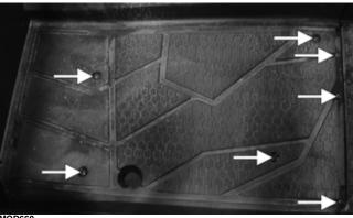
4. Gently lift the front portion of the rear floor up and remove from vehicle.
