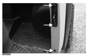
3. Remove the six fasteners on the occupant side securing the splash panel to the floor.
