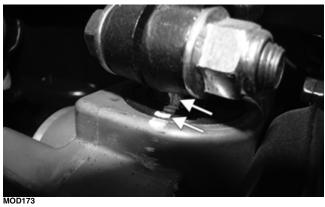
2. Reinstall the two cap screws on the occupant side and the one cap screw in the front left inner fender securing the EPS. Finger tighten only.
