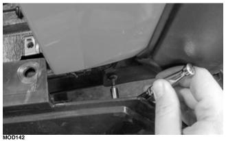
6. Install the three shouldered cap screws from the top of the side cover and the two shouldered cap screws from the bottom of the side cover.
