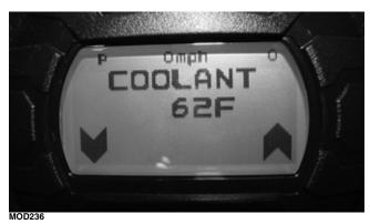
Display: Engine coolant temperature as measured by the ECT sensor.
