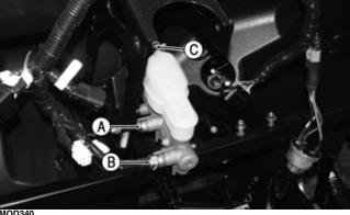
3. Remove the cotter pin and pivot pin from the yoke; then remove two cap screws securing the master cylinder assembly to the frame.
