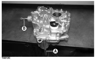
16. Using an appropriate seal installer, gently install a new plug over the pinion gear assembly so it fully seats past the chamfer — approximately 1.0-1.5 mm (0.04-0.06 in.) deep.
