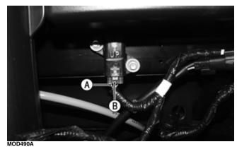
4. Tilt the sensor 60° or more to the left and right observing the meter. The meter should read 3.7-4.4 DC volts after approximately one second in the tilted position. If the meter readings are not as specified, the tilt sensor is defective.
