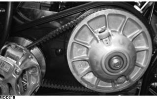
7. Rotate the driven clutch counterclockwise at least two times to verify belt is in the outermost portion of the sheave. Torque the cap screw to 60 ft lb (81.6 N-m) while holding the driven clutch with the Drive and Driven Clutch Holder Tool
