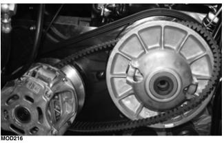
4. Push in on the outer portion of the driven clutch while rotating counterclockwise. Insert the cap screw with the washer bevel cup side toward the clutch and hand tighten with no tools.
