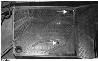
6. Gently lift the rear of the floor up and lift the floor out of the vehicle.
