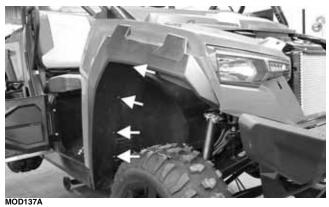
5. Gently pull on the front portion of the side panel; then install the cap screw securing the fender to the frame.
