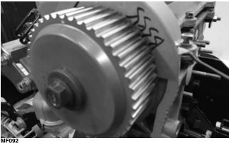
10. Tighten the camshaft drive pulley bolt to specifications; then install the camshaft drive belt making sure the camshafts are correctly timed to the crankshaft (see REMOVING AND INSTALLING CAMSHAFT DRIVE BELT in this section).
