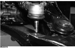
3. Measure the distance between shoulder of the tie rod shaft and the tie rod.
