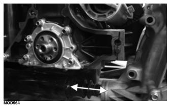
9. Remove the rear transaxle mount to frame cap screws and lock nuts (A); then gently slide the transaxle toward the front of the vehicle and remove the rear transaxle to transaxle mount cap screws and lock nuts (B); then being careful not to damage any items, gently remove the transaxle.
