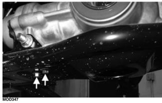
5. Remove the fill plug and pour the recommended amount of lubricant into the differential; then install the fill plug. Tighten to 16 ft-lb (21.8). Verify the location of the O-rings for the axles; then install the front axles by pushing the axle shaft (A) toward the inner CV joint housing (B) to release the "plunge" coupler; then while the axle shaft and the inner CV joint housing are pushed together install the axle to the differential. Repeat for the opposite side.
