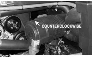
4. Loosen the clamp indicated and disconnect the snorkel from the housing; then clean and inspect the inside of the snorkel; then remove the primary air filter element; then wipe the inside of the housing to remove dirt and debris.
