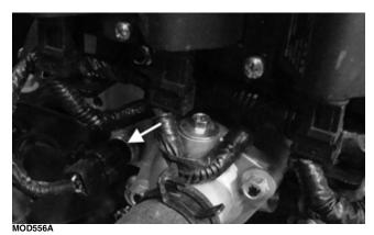
2. Set the meter selector to the OHMS position; then connect one lead to an outer spade terminal; then connect the other lead to the other outer spade terminal; then suspend the sensor and a thermometer in a container of cooking oil; then heat the oil.
