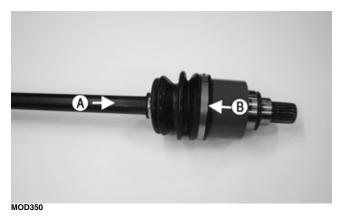
■NOTE: To ensure proper axle seating, give it a light pull; the axle should remain "clipped" in place.
