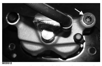
4. Compress the caliper holder against the caliper (opposite the O-ring side) and remove the outer brake pad; then remove the inner brake pad.
