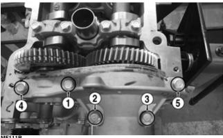
9. Install the camshaft drive and driven pulleys.
