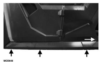
4. Open the front door; then remove the four cap screws securing the door; then remove the front door.
