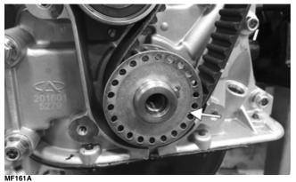
4. Loosen the cap screw securing the camshaft drive adjuster pulley; then remove the timing belt and replace if damaged in any way.
