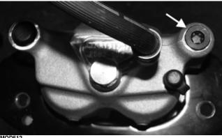
5. Place a new crush washer on the brake hose fitting and install it on the caliper. Tighten to 20 ft-lb (27.2 N-m).
