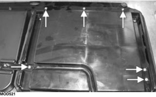
2. Position the center passenger seat back to the passenger seat backrest frame; then install the five flange nuts securing the center passenger seat back to the passenger seat backrest frame. Tighten to 4 ft-lb (5.4 N-m).
