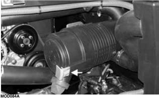
4. Connect the snorkel to the housing; then tighten the clamp securely.
