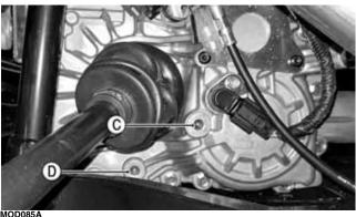
2. Drain the lubricant/fluid into a drain pan by removing the drain plugs from the right-side front differential (E) and transaxle (D).
