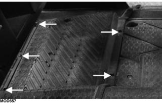
3. Gently lift the front portion of the center floor up and remove from vehicle.
