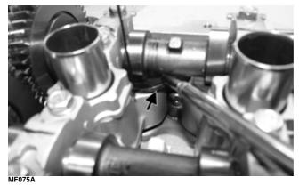
4. Read the number on the valve side of the adjustment shim placing a decimal point after the first number.
