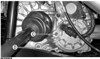
3. After the lubricant/fluid has been drained, install the drain plugs and tighten to 45 in.-lb (5.1 N-m) (front differential) and 16 ft-lb (21.8 N-m) (transaxle).
