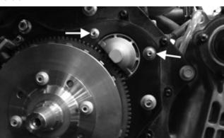
2. Secure the positive cable to the starter with the nut; then secure the start relay wire to the terminal.
