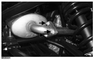
2. Lift the muffler assembly upward to clear the three holders underneath the muffler assembly.
