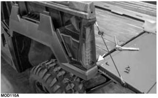
8. Start at the rear of the cargo box and tuck the outer side panel under the cargo box floor and work it into place from back to front.
