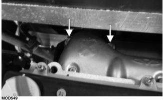
8. Install the fuel rail and injectors and secure with the two cap screws. Tighten to specifications.
