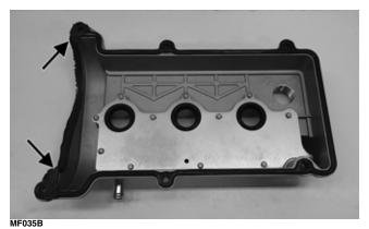
2. Install cap screws and tighten evenly to specifications; then install spark plug wires, spark plug cover, oil fill cap, and breather hose.
