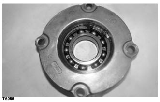
5. Using an appropriate bearing driver, press the bearing from the housing.
