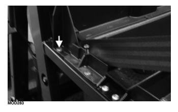
6. Disconnect the two electrical connections to the ECU (A) that is located in front of the engine air filter.
