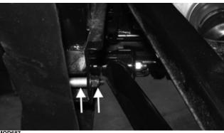
Remove the hook on the winch cable. Remove the two cap screws securing the winch fairlead; then remove the winch fairlead; then remove the four outer cap screws securing the bumper to the frame; then remove the bumper from the vehicle.
