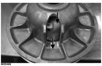
2. Install the roller pin with roller taking note of the flat spot that should be away from the sheaves; then align the holes for the new roll pin to be installed; then install the new roll pin. Repeat for the other side.
