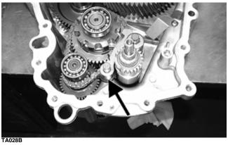
3. Remove the output gear assembly with bearings.
