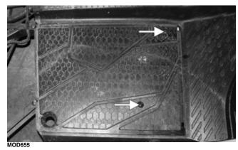
2. Install the two cap screws located near the front tires securing the splash panel to the floor on each side.
