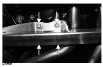
13. Using suitable clamps, clamp the areas indicated to minimize coolant leakage.
