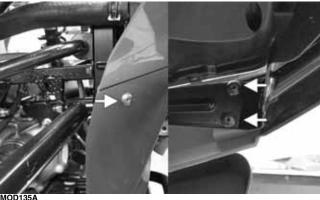
5. Install the upper grille and tighten the two T30 cap screws; then install the hood and secure the 1/4-turn locks.
