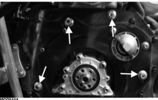
5. Install the two cap screws with blue Loctite #243 securing the backplate to the front mount and tighten to 51.7 ft-lb (70 N-m); then position the starter into place and install the two cap screws securing the starter to engine backplate; then tighten to 14.8 ft-lb (20 N-m).
