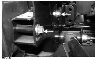
3. Remove the lower fascia-to-grille cap screw on each side.
