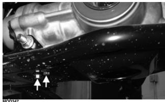
11. Reinstall the center floor section, and front skid plates.
