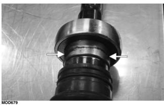
4. Coat all exposed driveshaft splines with molybdenum grease; then place the driveshaft into position.
