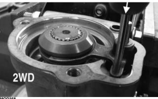
6. Align the splines of the output shaft to the internal splines of the coupler; then place the pinion housing onto the differential housing; then place the drive actuator bracket (A) into position; then secure the assembly with three cap screws and tighten to 22 ft-lb (29.9 N-m) (existing) or 28 ft-lb (38.1 N-m) (new differential housing).
