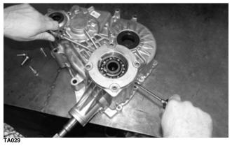
If the pinion shaft or bearing are being removed, use an awl and mallet to pry the front output seal off the case.
