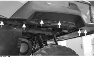
2. Remove screw (A); then flex the cargo box fender away from the cargo box to access and remove screw (B).
