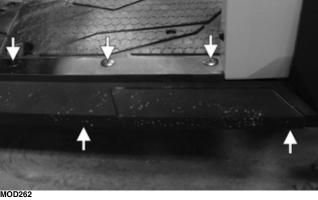
3. Gently pull on the front portion of the side panel; then remove the cap screw securing the fender to the frame.
