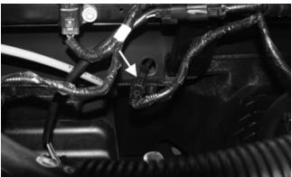
3. Buckle the driver's seat belt. On the switch side of the connector, connect one meter lead to one pin and the other meter lead to the opposite connector pin.
