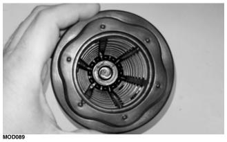
7. Remove and inspect the safety filter.
