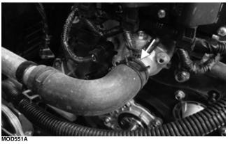
3. Located below the coils. Remove the two cap screws securing the thermostat housing.
