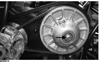
6. Remove the belt by pulling it over the driven clutch and rotating the driven clutch.
