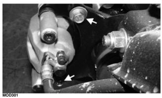
B. Remove the pads from the caliper; then install the new brake pads.
