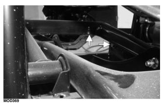
6. Remove the lower A-arm cap screws and lock nuts; then remove the lower A-arm.
