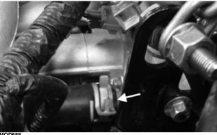
15. Remove the coolant sensor connector from the coolant sensor; then disconnect the coil connectors from the coils; then remove the engine oil pressure switch connector from the engine oil pressure switch that is located near the engine oil filter; then remove the engine ground located above the engine oil pressure switch.
