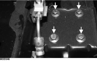
3. Remove the drive belt, drive and driven clutches; then remove the clutch cover housing; then remove the flywheel housing, crankshaft position sensor bracket with crankshaft position sensor, PTO stub shaft, and flywheel.
