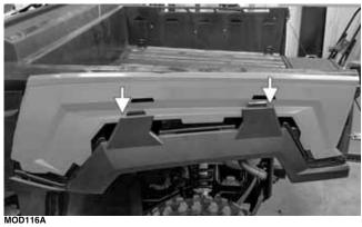
7. With a suitable pry bar, lift up on the inner cargo box floor near the rear corner.
