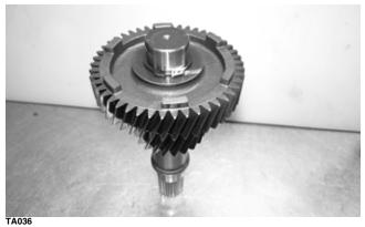
3. Inspect the shaft gear teeth for nicks, cracks, chips, or signs of wear. If any are present, the shaft must be replaced.
