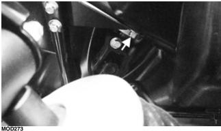
3. Align the U-joint of the steering tilt assembly to the input shaft of the EPS; then reinstall the two cap screws and nuts securing the steering tilt assembly. Tighten to 16 ft-lb (21.8 N-m).
