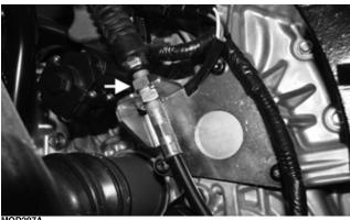
3. From under the dashboard, guide the shift cable into the bracket and install as shown; then secure the cable end to the shift lever using a new locknut. Tighten to 6 ft-lb (8.2 N-m) Tighten the shift cable nut to 20 ft-lb (27.2 N-m).
