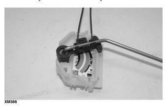
■NOTE: Inspect the float for any damage or leaking by submerging in water and looking for any air bubbles. Replace if damaged.
