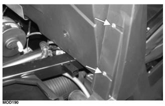
2. Reinstall the three cap screws from inside the behind-the-seat storage box panel.
