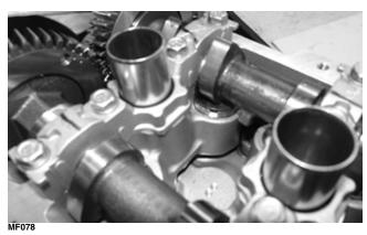
3. Remove the camshaft drive pulley; then remove the five cap screws securing the drive-end camshaft bearing housing and remove the housing.
