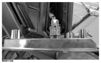
4. Install the new assembly, making sure to connect the harness.
