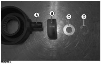
4. Install the spring into the clutch assembly with the spring tab in the clutch groove.
