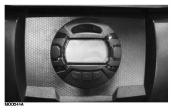
To install the gauge, connect the multi-pin connector and press the gauge into the dash.
