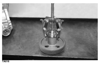
2. Inspect the gear teeth for nicks, cracks, chips, or signs of wear. If any are present, the gear must be replaced.
