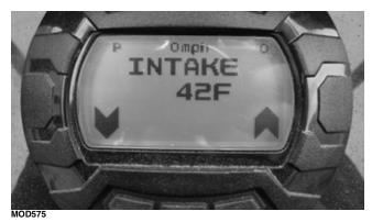
Display: Intake air temperature as measured by the Temperature Manifold Absolute Pressure (TMAP) sensor.
