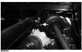
5. Disconnect the U-joint from the rack and pinion; then remove the rack and pinion from the passenger side.
