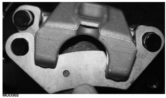
C. Secure the caliper holder to the knuckle with new "patch-lock" cap screws. Tighten to 45 ft-lb (61.2 N-m); then install the Torx head plug to the caliper.
