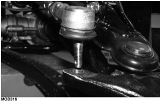
3. Remove the cap screw and lock nut securing the U-joint to the rack and pinion.
