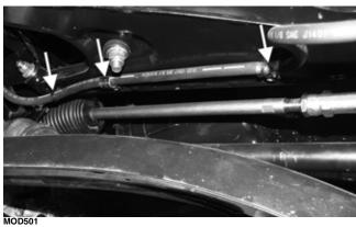
3. Remove the cotter pin and castle nut securing the tie rod end to the knuckle; then remove the tie rod end from the knuckle.
