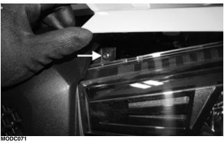
4. Install the two cap screws securing the inner portion of the front fenders and the grille.
