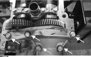
4. Loosen but do not remove the cap screws securing the camshaft bearing housings to the cylinder head.
