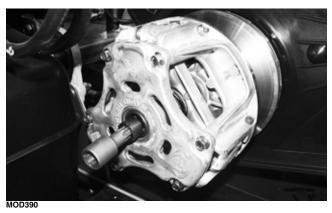
8. Lightly coat the threads and the end of the Drive Clutch Puller Tool with grease. Insert the Drive Clutch Puller Tool into the drive clutch. Tighten the Drive Clutch Puller Tool to remove the drive clutch.
