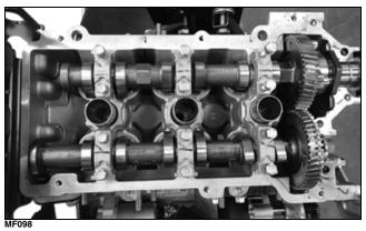
5. Use a sharp pick or small screwdriver to rotate the valve bucket until the notch is accessible; then lift the adjuster shim and remove using a small magnet or needle-nose pliers.
