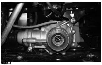
Remove the upper differential mounting bracket cap screws; then remove the upper differential mounting bracket.
