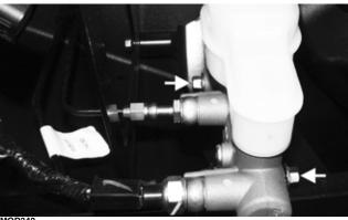
4. Remove the master cylinder. Discard the three crush washers.
