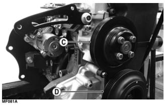
14. Install the serpentine belt and tighten as required.
