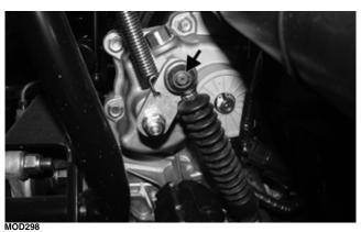
5. Loosen the adjuster nut; then remove the shift cable from the bracket. Remove any cable ties securing the shift cable to the chassis noting their location; then remove the shift cable.
