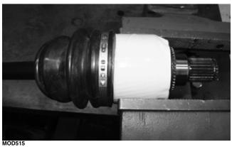
3. To disengage the axle from the CV joint, sharply pull back on the axle; then slide the boot off of the axle.
