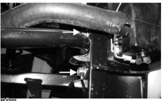
2. Position the sway bar link into the upper A-arms with the four bushings as shown; then using a wrench on the flat spot (A) of the sway bar link, install new sway bar link lock nuts (B). Tighten so there are 1-2 threads exposed on the upper sway bar link and 5-6 threads exposed on the lower sway bar link. Repeat for other side.
