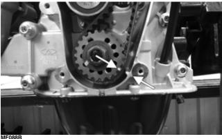
11. Install the camshaft drive belt guide with the tapered circumference directed away from the drive pulley.
