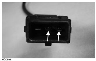
3. The meter reading must be 774-946 ohms at  $20^{\circ}$  C ( $68^{\circ}$  F).
