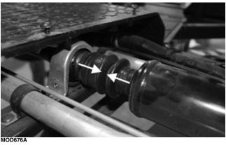
6. Install the carrier bearing cap screws and lock nuts; then tighten securely.
