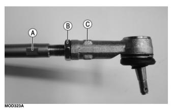
3. Place the outer tie rod ends into the knuckles and secure with the castle nuts (B) (coated with red Loctite #271). Tighten to 32 ft-lb (43.5 N-m); then install new cotter pins (A) and spread the cotter pins.
