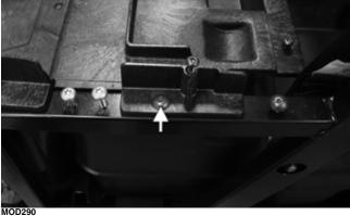
3. Remove the 13 cap screws securing the rear floor to the frame.
