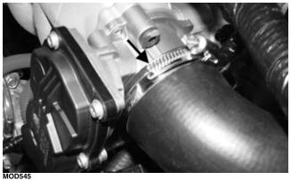
10. With tape or other suitable means, plug the intake for the engine to prevent foreign debris from entering.
