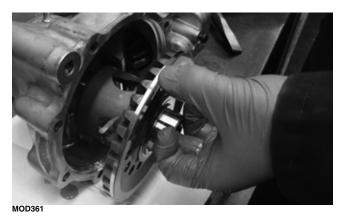
**Disassembling Pinion Gear**
