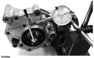
6. Zero the dial indicator; then while holding the pinion stationary, rock the ring gear assembly forward and back and record the backlash. Backlash must be 0.011-0.015 in. If backlash is within specifications, proceed to Ring Gear End-Play. If backlash is not within specifications, increase shim thickness to increase backlash or decrease shim thickness to decrease backlash.
