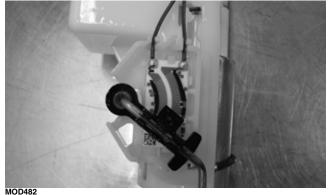
Connect the blue wires using the supplied splice connectors from the fuel level sensor kit. Secure the wires.
