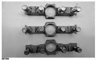
9. Inspect the camshaft bearing journals and caps for scoring, flaking, galling, or signs of heat damage. If damage is present, the cylinder head will have to be replaced (see REMOVING AND INSTALLING CYLINDER HEAD in this section).
