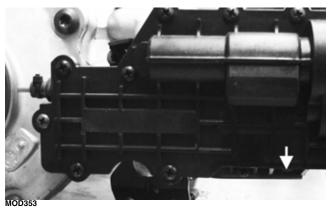
4. Loosen but do not remove the mounting cap screw at the front of the actuator; then slide the actuator to the rear enough to clear the slotted mounting tab and the selector shaft.
