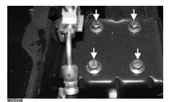
10. Install the upper differential mounting cap screw with a new lock nut. Tighten to 45 ft-lb (61.2 N-m); then tighten the lower differential mounting cap screws to 16 ft-lb (21.8 N-m).
