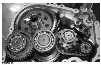
11. Apply a coat of Loctite #5699 to the case; then ensuring the shift shaft (O-ring lightly coated with grease) and shift rail are correctly seated; install the axle lock collar (A) on the cover and the axle lock solenoid (B); then install the cover.
