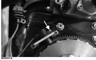
6. Remove the flywheel; then with a suitable lift put a slight upward tension on the engine; then with a suitable strap or lift put a slight upward tension on the transaxle.
