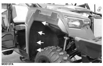
5. Remove the three cap screws indicated.
