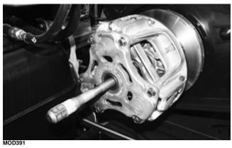
3. Near the engine PTO, remove the retaining ring securing the inner clutch cover to the engine; then near the transaxle input shaft remove the four cap screws securing the inner clutch cover to the transaxle; then remove the inner clutch cover.
