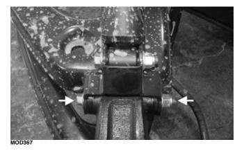
3. While holding the drive axle stationary, use a rubber mallet, and tap the end of the axle free from the knuckle assembly; then pull the top of the knuckle out and down until it is free of the drive axle; then repeat for the other side.
