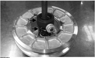
5. Place the cam in the movable sheave making sure the "X" timing marks are aligned.
