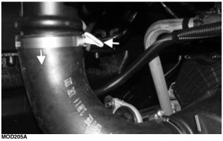
4. Remove the six clamps securing the clutch cover; then remove clutch cover.
