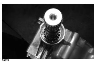
■NOTE: To determine the appropriate shim, start with the thickest shim and install the snap ring. If the snap ring will not fit in the groove, remove the shim and install the next size smaller shim. Continue until the snap ring can be installed.
