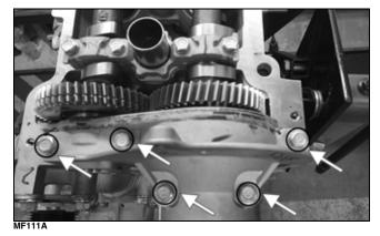
4. Install a 5 mm x 80 cap screw in the hole next to the pinned hole on the intake camshaft drive gear and tighten to secure the master and slave gears in position; then rotate the camshafts to relieve the valve spring pressure (approximately 1/3 turn).
