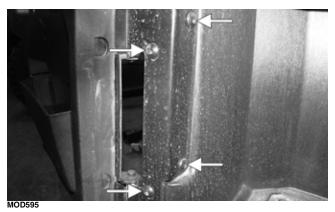
4. Install the three cap screws securing the side panel to the floor; then install the four cap screws underneath the side panel.
