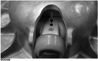
3. Install the rollers (B), washers (C) and e-clips (D) onto both of the spider arms (A).
