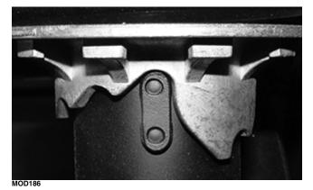
■NOTE: Before attempting to adjust suspension, clean dirt and debris from the sleeve and remove load from the suspension; then use the spanner wrench to adjust the sleeve to the desired position.
