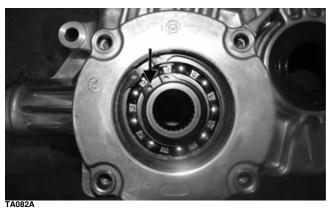
3. With the aid of an assistant and using an appropriate driver, remove the gear.
