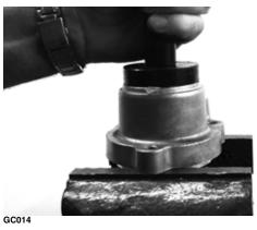
3. Lubricate the input shaft with High-Performance #2 Molybdenum Disulfide Grease packing the splines; then assemble allowing excess grease to freely escape. Grease the pinion housing seal; then install the input shaft into the pinion housing and secure with a new snap ring.
