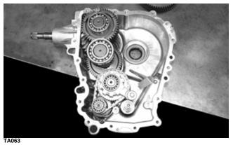
5. Install the output gear. Use slight force to seat it and ensure the gear teeth engage with the intermediate shaft.
