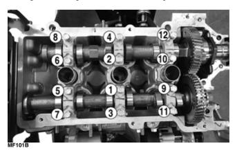
■NOTE It is recommended that the cap screws be tightened in several increments to allow the camshafts to be evenly seated in the camshaft bearings.
