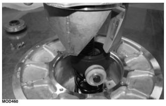
3. Remove the spider and driven spring from the driven clutch assembly.
