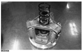
3. Remove the lock nuts (C) from the cam arm pivot pins (B); then remove the pins and three cam arms (A).
