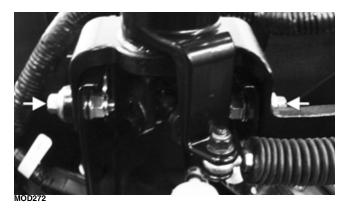
4. Reinstall the input shaft cap screw and nut to the EPS; then reinstall the output shaft cap screw and nut of the EPS. Tighten both to 24 ft-lb (32.6 N-m).
