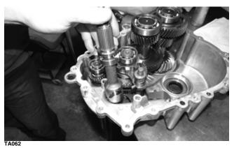
4. Pinch the forks together and slide the rail into position in the case.
