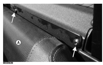
3. Remove the two cap screws at the bottom of the seat back; then remove the seat back assembly.
