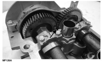
15. Install the camshaft bearing caps in their proper location and orientation: then secure with the cap screws tightened to specifications in the sequence shown.
