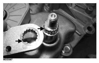
■NOTE: Ensure the transaxle is in neutral by turning the input shaft (A). It should turn freely and the front output shaft (B) should not turn.
