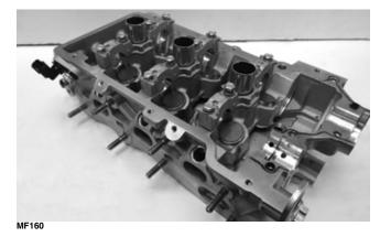
8. Inspect the camshaft bearing surfaces in the cylinder head and the bearing caps for signs of scoring, galling, or heat damage. If damaged, the engine must be replaced.
