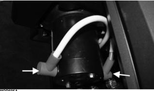
3. Remove the passenger-side bumper bracket; then gently slide the winch out the passenger side of the vehicle.
