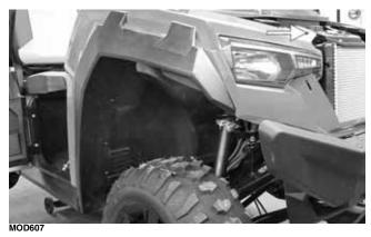
7. With the fender removed from the vehicle, remove the four cap screws on the inside of the fender; then remove the fender flare from fender taking note of the four tabs on the fender flare.
