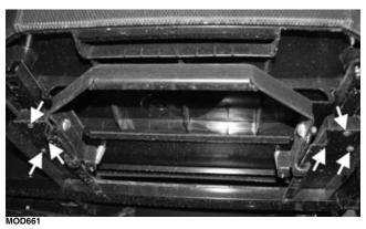
2. Lift the seat adjustment lever; then move the seat assembly toward the front of the vehicle to clear the rear mounting channel.
