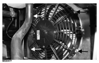
2. Connect the radiator fan electrical connection.
