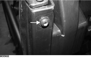
6. Remove the three cap screws securing the side panel to the floor; then gently remove side panel.
