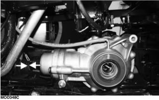
8. Install the lower differential mounting cap screws. Do not tighten at this time.
