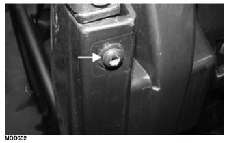
3. Position the front door into position; then install the four cap screws securing the door.
