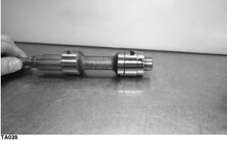
4. Check the detent star (A) and shift drum gear (B) for nicks, cracks, chips, or signs of wear. If any are present, the detent star must be replaced.
