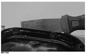
3. Thoroughly clean all gasket and sealing materials from the mating surfaces; then invert the oil pan on a flat surface and check for irregularities in the perimeter of the oil pan. Straighten as required.
