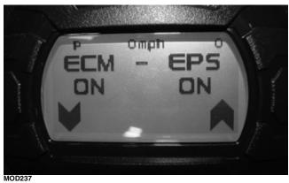
Display: Communication from the Engine Control Module (ECM) and the Electronic Power Steering (EPS). "ON" is receiving communication and "OFF" is not receiving communication.
