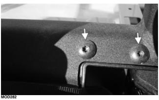
4. Reinstall the passenger seat back hinge; then reinstall the 11 cap screws securing the passenger seat back hinge.
