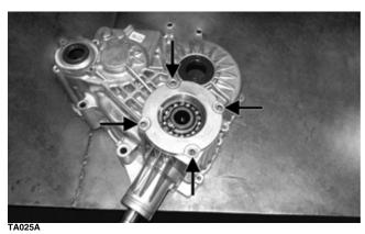
8. Pry the pinion gear assembly to remove it from the case. Account for the shim.
