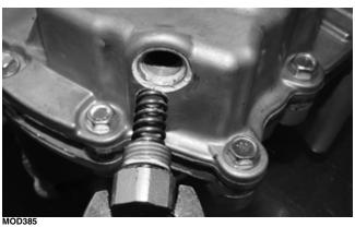
14. Align the shaft and the alignment pin on the gear position switch to the transaxle case; then install the gear position switch. Secure with the wave washer and snap ring.
