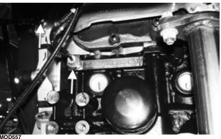
16. Remove the wires going to the alternator; then remove the temperature/manifold absolute pressure (TMAP) sensor connector from the temperature/manifold absolute pressure (TMAP) sensor.
