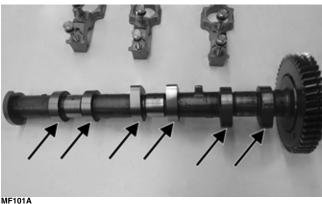
11. Inspect the camshaft drive gears for excessive wear, chipped or missing teeth, and security to the camshafts. Replace as required.
