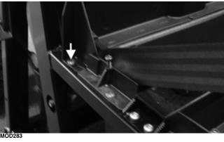
Reinstall both seat belt guides; then reinstall the two cap screws on each seat belt guide; then connect the seat belt electrical connector.
