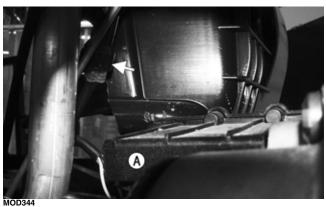
4. Remove the outer tie rods from the knuckle; then remove the lower and upper ball joint cap screws taking care not to strip the threads on the ball joint shaft; then, using a rubber mallet, tap the end of the axle and free it from the knuckle assembly. Repeat for the other side.
