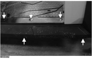
7. Located in the front of the inner fender, install the two cap screws securing the fender, fender flare and grille to the headlight bracket. Install the upper hood, mid/upper dashboard and hood; then adjust doors as needed.
