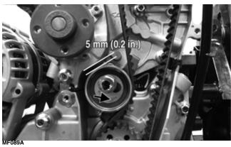
10. Rotate the crankshaft clockwise two turns, aligning the timing marks again; then loosen the tensioner cap screw and apply pressure to the arm so as to obtain a belt deflection of 5 mm (0.2 in.) midway between the pulleys when applying a force of 20-30 N (4-6 lb.).
