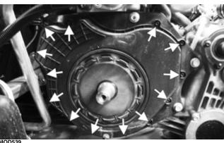
3. Install the inner clutch cover; then near the engine PTO, install the retaining ring securing the inner clutch cover to the engine; then near the transaxle input shaft, install the four cap screws securing the inner clutch cover to the transaxle and tighten to 8 ft-lb (10.9 N-m).
