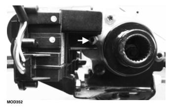
■NOTE: It is important to tighten this cap screw while the others are loose to ensure proper seating of the actuator.
