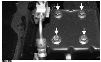
4. Remove the two cap screws and lock nuts securing the carrier bearing to the frame.
