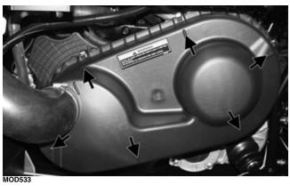
Connect clutch air inlet to snorkel portion; then install the clamp that holds the snorkel portion to the air inlet.
