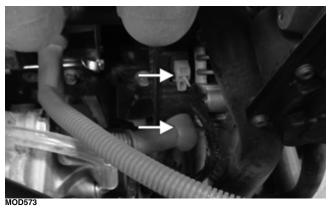
3. Loosen the alternator adjuster cap screw (A) and the pivot bolt (B); then remove the serpentine belt.
