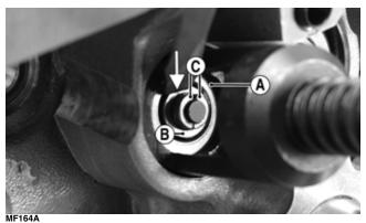
4. Remove the collets (C) from the valve stem; then release the spring compressor and account for valve spring (A), sleeve (B), valve spring retainer (D), valve stem seal (E), valve spring seat washer (F), and valve (G).
