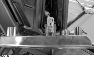
5. Install screw (A) first; then flex the cargo box fender away from the cargo box to access and install screw (B).
