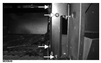
5. Remove the cap screw near the center ROPS-tochassis connection.
