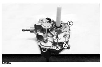
■NOTE: Use a suitable bearing seal protection tool when driving the bearing and gears into the lower half of the transaxle.
