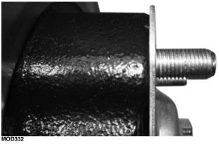
4. Secure the brake calipers to the knuckle with two new "patch-lock" cap screws tightened to 45 ft-lb (61.2 N-m).
