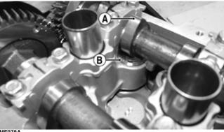
4. Using a suitable feeler gauge, check clearance between the camshaft and the valve bucket recording the value when a slight drag is felt when inserting and retracting the gauge blade.
