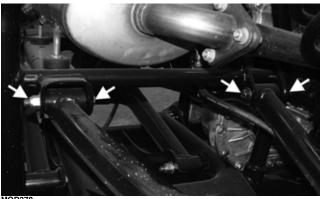
■NOTE: When removing a lower A-arm it is required to lift the opposite lower A-arm in order to have access to the cap screws. This is best accomplished by removing the lower shock mount cap screw for the opposite A-arm and using a suitable strap to lift the A-arms.
