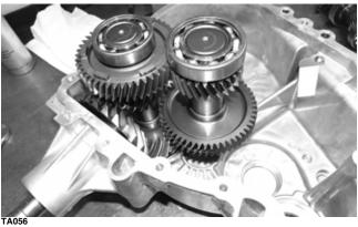
2. With the aid of an assistant and with the gear forks in position, install the input shaft and reverse shaft with chain as an assembly.
