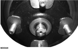
6. Using Hub Retaining Wrench, secure the hub assembly with the nut. Tighten to 250 ft-lb (339 N-m).
