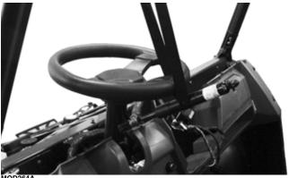
Remove the key switch locking nut by turning counterclockwise; then push the key switch through hole to clear the lower dashboard; then disconnect the electrical connectors on the left side of the dashboard.
