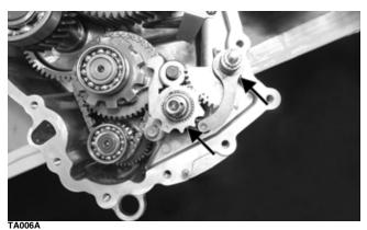
2. Remove the park pawl with dowel pin and account for the spring.
