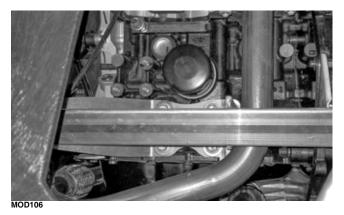
■NOTE: Clean up any excess oil after removing the filter.
