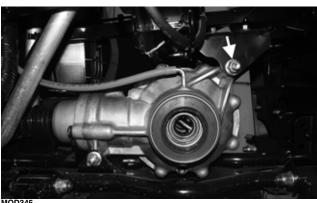
11. Install the two cap screws underneath the front differential; then tighten to 16 ft-lb (21.8 N-m); then install the cargo box; then install both rear drive axles; then install both rear inner fenders.
