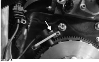
4. Using a suitable tool to hold the PTO/flywheel in place, remove the four cap screws securing the PTO stub shaft to the flywheel; then remove the six cap screws securing the flywheel to the crankshaft.
