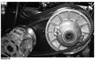
2. Push in on the outer portion of the driven clutch while rotating counterclockwise. Insert the cap screw with the washer bevel cup side toward the clutch and hand tighten with no tools.
