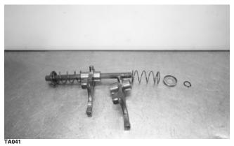
2. Inspect the rail for nicks, cracks, chips, or signs of wear. If any are present, the rail must be replaced.
