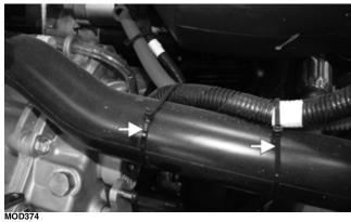
8. Connect the shift cable to the transaxle. Then remove the suitable strap that was putting a slight upward tension on the engine.
