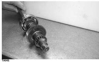
3. Inspect the shaft gear teeth for nicks, cracks, chips, or signs of wear. If any are present, the shaft must be replaced.
