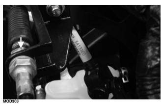
Remove the E-clip securing the cable end to the shift arm stud.
