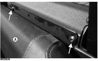
3. Install the rear driver-side seat bottom.
