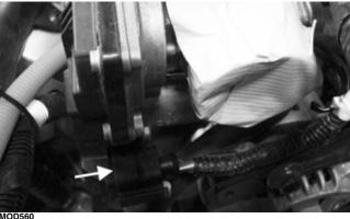
12. Install the wires going to the alternator; then install the temperature/manifold absolute pressure (TMAP) connector to the temperature/manifold absolute pressure (TMAP) sensor.
