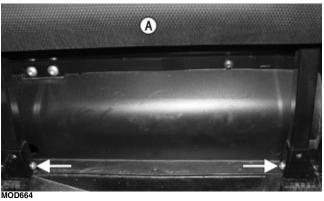
2. Install the two cap screws at the top of the seat back (A).
