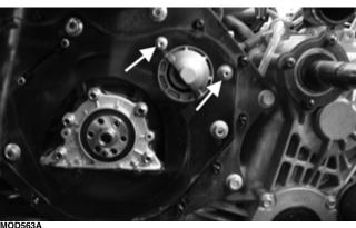
6. Install the spacers for the transaxle to engine mount; then install the two cap screws to secure the transaxle to engine. Tighten to 75 ft-lb (102 N-m).
