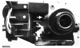
3. Remove the mounting cap screw from below the actuator.
