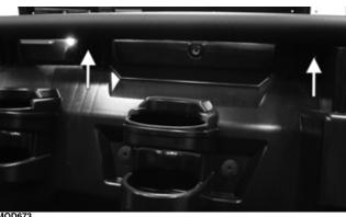
4. Reinstall the six cap screws that secure the rear panel to the center ROPS.
