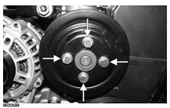
4. Remove the three cap screws securing the water pump; then remove the water pump.
