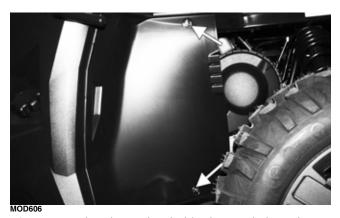
Loosen the clamp that holds the snorkel portion to the air inlet; then disconnect snorkel portion from air inlet.
