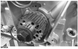
Inspect belt tensioner for excessive wear, binding, or rough bearing feel. Replace as necessary.
