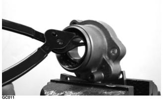
2. Install the input shaft seal making sure it is fully seated in the edge of the housing.
