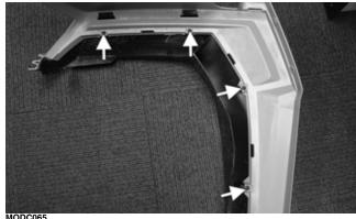
2. Place the fender into position; then install the two cap screws on the top portion of the fender.
