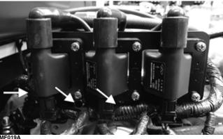
12. Connect the coolant temperature connector (4) to the coolant temperature sensor.
