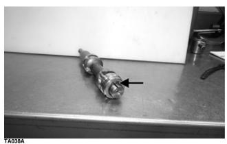
2. Inspect the cam groove for signs of wear. If present, replace the cam.
