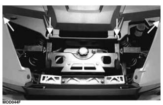
2. Remove the cap screws located next to each cup holder; then the cap screws in the middle; then remove mid/upper dash.
