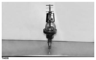
Inspect the gear teeth for nicks, cracks, chips, or signs of wear. If any are present, the gear must be replaced.
