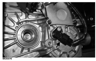
6. Remove the two cap screws securing the transaxle to the engine. Account for the spacers.
