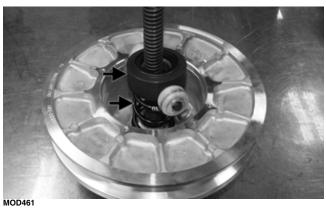
4. Remove the E-clips (D) on the end of both the spider arms (A); then remove the rollers (B) and washers (C) from both spider arms.
