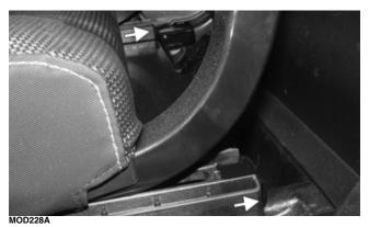
2. Install the six cap screws underneath the driver seat rails. Tighten to 2 ft-lb (2.7 N-m).
