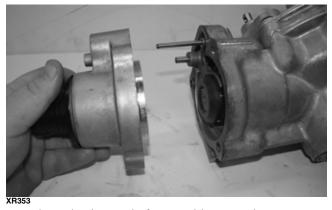
7. Place the input shaft assembly onto the gear case housing; then with the actuator bracket in place, secure with the existing cap screws. Tighten to 22 ft-lb (29.9 N-m).
