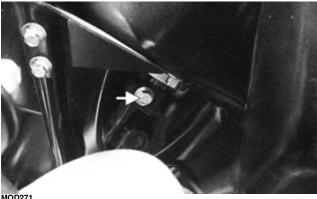
4. Remove the two cap screws securing the steering tilt assembly; then pull the U-joint off of the input shaft of the EPS; then secure the steering tilt assembly out of the way.
