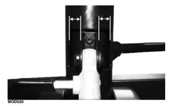
■NOTE: If the distance on each side of the upper tilt steering wheel adjuster bracket and the shifter housing is the same and the vehicle does not properly engage Park or Low, shift cable replacement may be required.
