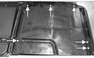
2. Remove the five flange nuts securing the passenger seat backrest to the passenger seat backrest frame; then remove the passenger seat backrest from the passenger seat backrest frame.
