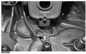
15. Install the bell crank being sure to correctly align the splines of the bell crank and shift shaft and secure with a new lock nut. Tighten to 15 ft-lb (20.4 N-m).
