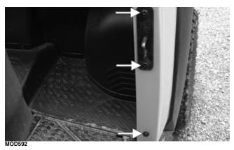
6. Remove the two remaining cap screws on the top portion of the fender; then remove fender. If fender flare removal is desired, continue to step 7.
