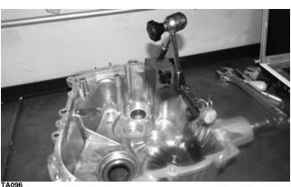
5. While pushing in on the front output shaft, and while rocking the shaft back and forth, note the maximum backlash reading on the gauge.
