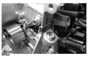
7. Rotate the camshaft driven pulley to align the timing mark (F) on the pulley with the reference mark (G) on the camshaft retainer housing.
