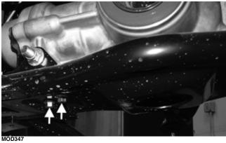
3. Remove the upper mount cap screw and lock nut for the front differential; then remove the four cap screws securing the upper differential mount; then remove the upper differential mount.
