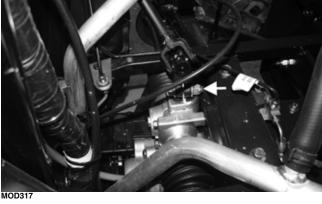
4. Remove the four cap screws and lock nuts securing the rack and pinion bracket to the frame.
