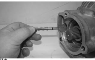
5. Place the dowel pin into the differential housing; then install a new gasket. Place the coupler onto the shift fork; then simultaneously engage the shift fork to the shuttle shaft and the internal splines of the coupler to the splines of the pinion gear shaft; then verify the shift fork moves freely from 4WD to 2WD to 4WD by pushing down on the shift fork shaft and then releasing.
