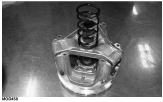
3. Align the match marks (X) and install the clutch cover and secure with six cap screws. Tighten using a crisscross pattern to 110 in-lb (12.4 N-m).
