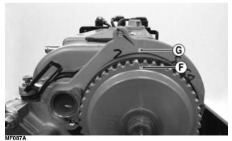
8. Rotate the crankshaft to align the timing mark (H) on the drive pulley to the reference mark (I) on the oil pump housing.
