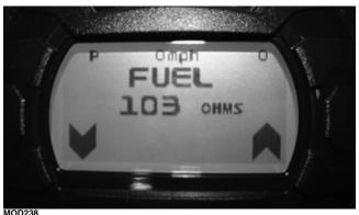
Display: Fuel level signal from the fuel level sensor.
