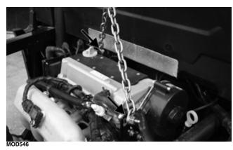
5. Remove the nylon straps and disconnect the electrical connections to the transaxle.
