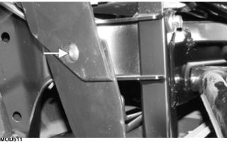
2. Position the tow hooks into place; then install the two cap screws behind each tow hook. Tighten to 20 ft-lb (27.2 N-m).
