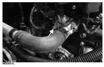
4. Gently remove the thermostat housing away from the engine. Remove the thermostat. Account for the thermostat housing gasket.
