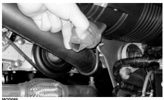
3. Pull out on the orange air filter housing cover lock; then turn the air filter housing cover counterclockwise to access the filter.
