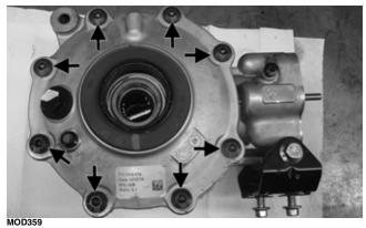
3. Using a plastic mallet, tap lightly to remove the differential cover. Account for an O-ring (A) and note the location of any shims.
