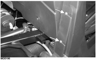
2. Remove the three cap screws from inside the behindthe-seat storage box panel.
