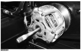
Remove the Drive and Driven Clutch Holder Tool, drive clutch, driven clutch, and Drive Clutch Puller Tool.
