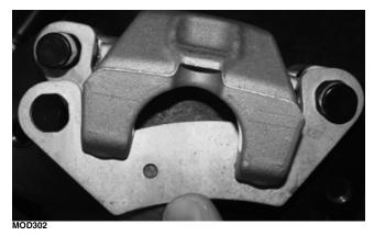
5. Remove the brake hose from the caliper and close the bleed screw; then remove the caliper mounting bracket from the caliper.
