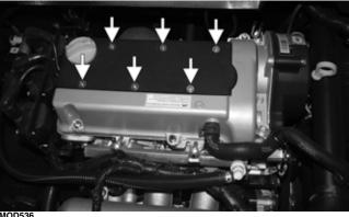
3. Remove spark plug wires; then remove six cap screws securing valve cover to the cylinder head.
