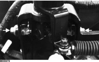
5. Remove the two cap screws on the occupant side and the one cap screw in the front left inner fender securing the EPS; then gently remove the EPS taking note that the output shaft should slide away from the U-joint.
