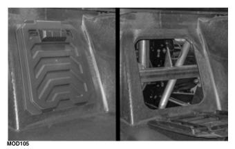
3. Tilt the cargo box to the dump position; then loosen the oil fill cap. Be careful not to allow contaminants to enter the opening.
