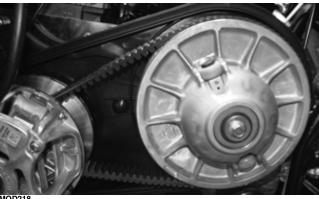
5. Rotate the driven clutch counterclockwise at least two times to verify belt is in the outermost portion of the sheave. Torque the cap screw to 60 ft-lb (81.6 N-m) while holding the driven clutch with the Drive and Driven Clutch Holder Tool
