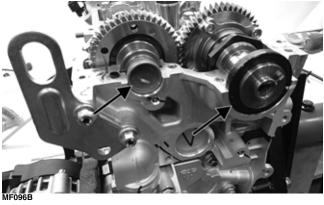
7. Make sure the cap screw from step 4 is properly installed; then carefully lift the camshafts from their respective journals using caution not to lift unevenly causing binding or galling of the camshaft bearing surfaces.
