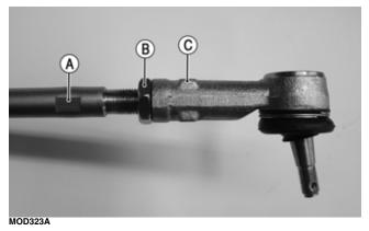
2. Hold the outer tie rod with a wrench at the location indicated (C) and tighten the lock nut (B).
