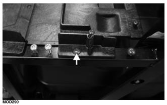
3. Install the 13 cap screws securing the rear floor to the frame.
