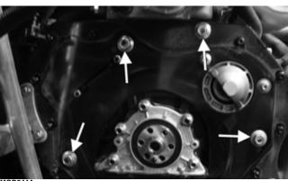
3. Install the two cap screws with blue Loctite #243 securing the backplate to the front mount and tighten to 51.7 ft-lb (70 N-m); then position the starter into place and install the two cap screws securing the starter to engine backplate; then tighten to 14.8 ft-lb (20 N-m).
