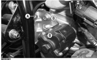
3. Lightly coat the splines of the driveshaft with grease; then couple the driveshaft to the transaxle by gently sliding the front differential with the driveshaft toward the rear of the vehicle. Verify the O-rings and boot are intact for the coupler
