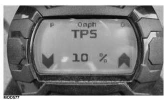
Display: Throttle position sensor percentage as measured by the throttle position sensor from the throttle body.
