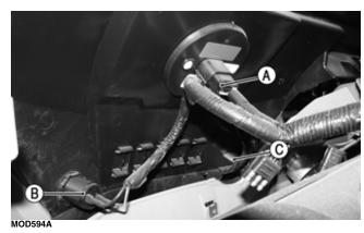
2. Gently position the dashboard, taking note of the tabs on each side that must be positioned at an angle; then place dashboard over cup holders.
