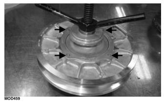
2. Gently release the suitable compressor; then remove the cam from the driven clutch assembly.
