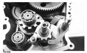
10. Install an appropriate bearing seal protector tool onto the output shaft.
