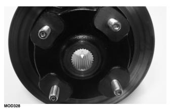
2. Install the hub assembly onto the axle.
