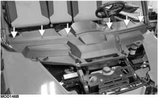
3. Gently lift the mid/upper dashboard above the cup holders on each side. Take note of the tabs on each side that must be lifted vertically at an angle.
