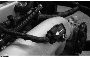
17. Disconnect the gas line from the injector rail; then disconnect each injector connector from the injector; then disconnect the electronic throttle control (ETC) connector from the ETC.
