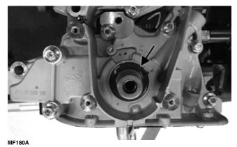
3. Using a new gasket (C), place the oil pump pick-up assembly (B) into position; then applying a drop of red Loctite to the threads of the cap screws (A), secure the oil pump assembly to the oil pump and engine block. Tighten securely.
