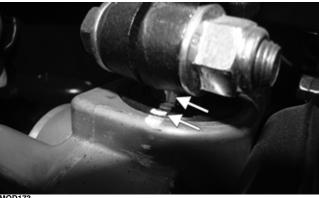
3. Remove the input shaft cap screw and nut of the EPS; then remove the output shaft cap screw and nut of the EPS.
