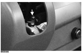
4. Remove the two cap screws securing the adjuster bracket to the bottom of the steering housing.
