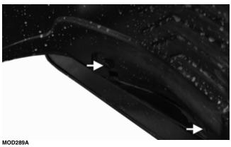
3. Install the six fasteners on the occupant side securing the splash panel to floor.
