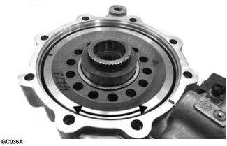
3. Install the existing shim or a 0.063 in. shim on the cover side of the ring gear; then place the assembled gear case cover onto the gear case and secure with three cap screws. Tighten evenly using a crisscross pattern.
