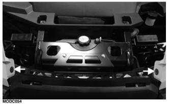
2. Gently lift up on the front fenders where it meets the grille to gain access to the upper headlight cap screw; then remove the upper headlight cap screw; then repeat for other side.
