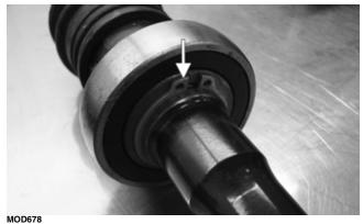
3. Remove each set screw and place one drop of red Loctite #271 on each; then install and tighten securely.
