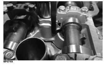
3. Firmly holding the bucket retainer and rotate the crankshaft so as to position the camshaft lobe high point away from the valve bucket; then, using a small screwdriver and magnet, tip the valve adjustment shim up and out of the valve bucket.
