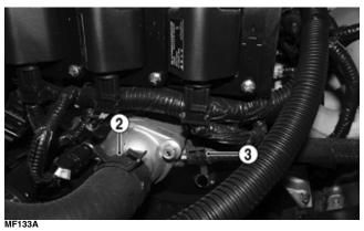
6. Remove the cap screws securing the exhaust pipe to the exhaust manifold and separate the exhaust pipe from the manifold. Account for the gasket.
