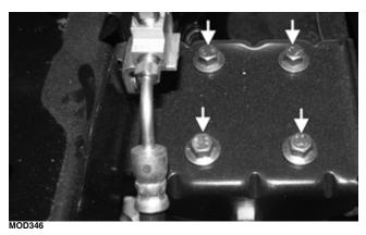
11. Remove the lower differential mounting bracket cap screws.
