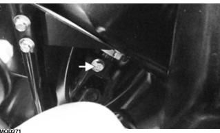
5. Reconnect the EPS electrical connection with dielectric grease on the terminals; then tighten the cap screws from step 2 to 16 ft-lb (21.8 N-m); then reinstall the dash lower, dash upper, upper hood, and hood; then reconnect the battery.
