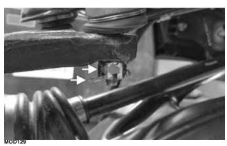
4. Remove the cap screws securing the ball joints to the knuckle.
