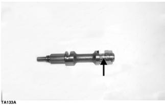
3. Check the shaft splines for nicks, cracks, chips, or signs of wear. If any are present, the shift drum must be replaced.
