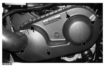
5. Using the Drive and Driven Clutch Holder Tool to hold the driven clutch remove the cap screw securing the driven clutch.
