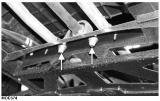
5. Gently pull the front driveshaft away from the rear driveshaft and account for the rubber bumper.
