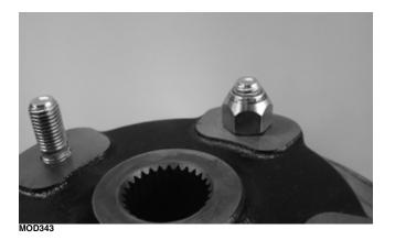
3. Using a socket and ratchet handle, tighten the nut until the stud is fully drawn into the hub.
