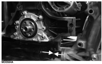
4. Clean the engine backplate; then apply black RTV silicone to the engine in the areas indicated; then position the engine backplate into place; then install the four cap screws securing the engine backplate to the engine and tighten to 51.7 ft-lb (70 N-m).
