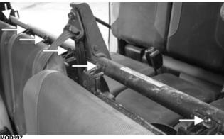
3. Remove the two cap screws behind the center seat; then remove the two cap screws behind the passenger seat.
