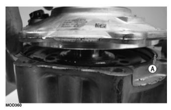
■NOTE: If the cover is difficult to remove, pry on the cover in more than one recessed location.
