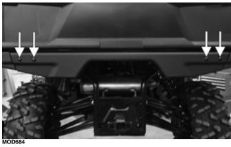
Remove the four cap screws and two lock nuts per bumper bracket; then discard lock nuts; then remove bumper brackets.
