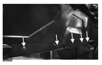
3. Reinstall the two cap screws behind the center seat; then reinstall the two cap screws behind the passenger seat.
