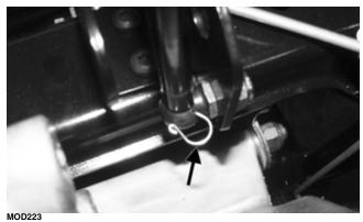
4. Remove lift support from mounting; then carefully lower the cargo box to the down position.
