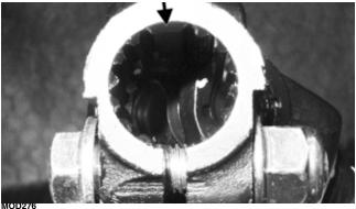
1. Align the steering rack with the marks; then reinstall the output shaft of the EPS into the U-joint going to the steering rack; then install the EPS into position.
