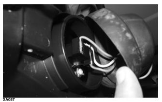
2. Press forward then up on the spring clip and swing the spring clip away from the bulb; then remove the bulb from the housing.
