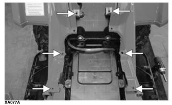
5. Place the PDM, SIG relay, and starter relay into their respective positions within the battery tray. Ensure the PDM locks into place. Connect the starter relay primary connector (B) and green ground wire connector (A).
