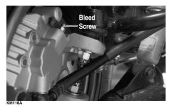
■NOTE: During the bleeding procedure, watch the reservoir sight glass very closely to make sure there is always a sufficient amount of brake fluid. Failure to maintain a sufficient amount of fluid in the reservoir will result in air in the system.
