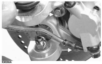
B. Remove the caliper from the disc; then compress the caliper holder and remove the brake pads.
