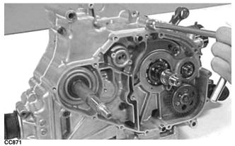
5. In a crisscross/case-to-case pattern, tighten the cap screws until the halves are correctly joined; then tighten to 8 ft-lb.
