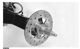
14. Install the hub nuts and tighten to 72 ft-lb; then install new cotter pins and bend as shown.
