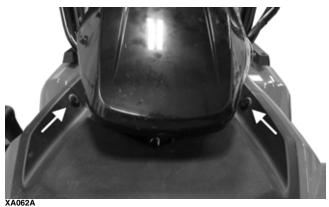
5. Remove the gas tank cap and two reinstallable rivets securing the gas tank cover. Slide the cover forward to remove.
