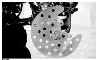
Remove the cotter pin and slotted nut securing the tie rod end to the knuckle; then remove the tie rod end from the knuckle.
