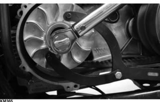
6. Install the centrifugal clutch housing and clutch collar; then secure with the flange nut and tighten to 40 ft-lb.
