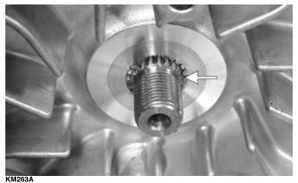
5. Install the starter ratchet on the crankshaft making sure to engage the splines; then secure with the flange nut and tighten to 68 ft-lb.
