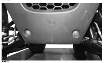
10. Remove the Allen-head screw securing the shift knob to the shift lever. Turn the steering wheel full left and remove the front body panel.
