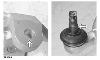
■NOTE: During assembly, new cotter pins should be installed.
