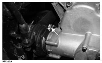
9. Connect the V-belt cooling boots to the V-belt housing and secure with the existing hose clamps.
