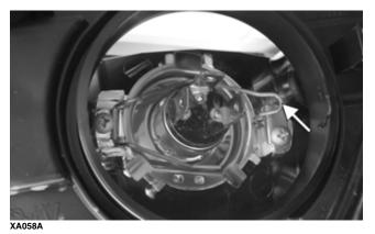
3. Install the new bulb into the housing; then secure with the spring clip.
