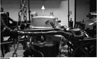
16. Remove the upper rear and lower rear engine through-bolts to free the engine/transmission; then raise the front of the engine/transmission sufficiently to allow the engine assembly to be moved forward enough to disengage the driveshaft.
