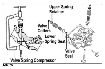
2. Remove the valve seal, valve springs, and the lower remaining spring seat. Discard the valve seal.
