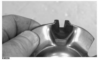
2. Inspect the face surfaces of the fixed and movable drive faces for grooving, nicks, or discoloration.
