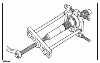
3. Apply oil to the secondary driven bevel gear shaft; then install the bearing into the case.
