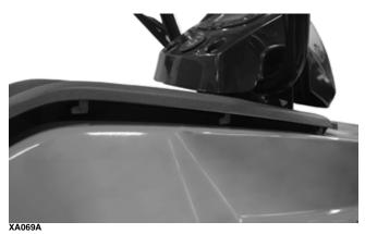
6. Remove the Phillips-head screws with lock nuts and three cap screws securing each footwell to the vehicle. Remove the footwells.
