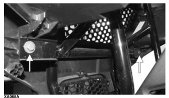
3. Secure the shift knob to the shift lever using the Allen-head screw. Secure the CVT intake tube using the two machine screws. Connect each headlight connector; then secure the connectors to the frame via the locking tabs.
