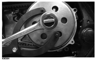
5. Remove the outer clutch housing; then remove the centrifugal clutch, driven pulley, and V-belt.
