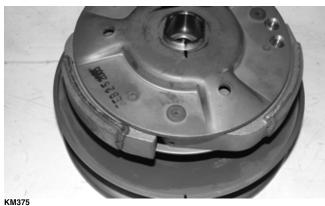
4. Remove the spring and spring seat; then remove the hub collar.
