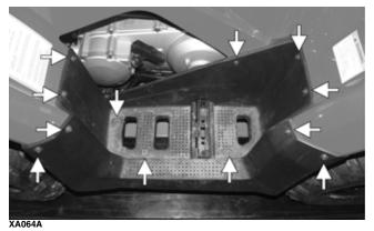
7. Remove the four cap screws securing the rear section of the front body panel to the frame; then remove the two cap screws securing the body panel to the gas tank.
