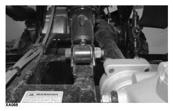
■NOTE: Support the swing arm with a block of wood or other support to allow removal of the cap screw.
