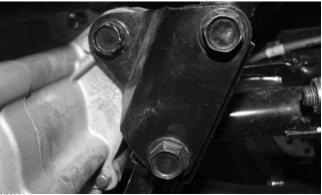
5. Install the front engine through-bolt; then tighten the engine mounting brackets to 16 ft-lb.
