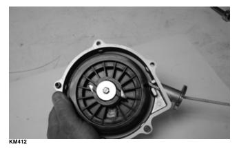
■NOTE: Increasing the rotations in step 10 will increase spring tension.
