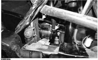
15. Install the air hose into the cylinder head.
