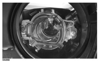
4. Connect the three-wire connector to the bulb; then install the rubber boot.
