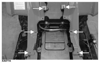
4. Remove the self-tapping screws securing the rear over-mold to the rear rack; then remove the four cap screws securing the rear rack to the frame. Remove the rack. Account for the four steel inserts installed into each rubber grommet.
