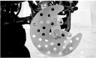
8. Connect the tie rod ends to the steering knuckle; then tighten the nut to 15 ft-lb and install a new cotter pin.
