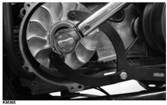
4. Hold the centrifugal clutch with a suitable holder; then remove the clutch retaining nut and clutch collar.
