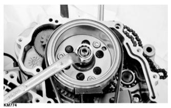
18. Install the flywheel puller and crankshaft protector; then remove the rotor/flywheel. Account for a key and the starter one-way clutch bearing.
