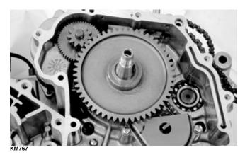
**NOTE:** Make sure the crankshaft and rotor/flywheel contact surfaces are clean and dry before installing the flywheel.
