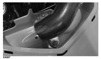
9. From within the front fascia, remove the two cap screws securing the fascia to the front bumper. From the front of the vehicle, remove the two cap screws securing the front of the fascia to the bumper.
