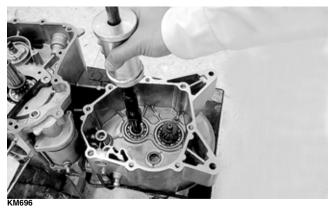
2. Replace any required bearings and seals in the secondary driven bevel gear shaft case. Apply oil to all seal lips.
