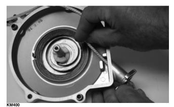
5. Align the inner hook of the spiral spring with the notch in the reel spacer.
