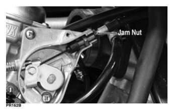
8. Disconnect the vent hose; then remove the carburetor.
