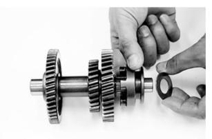
8. Install the low driven gear washer on the driveshaft; then install the low driven gear and thrust washer. Secure with a snap ring.
