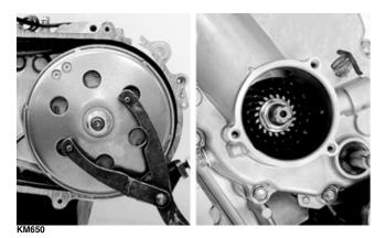
■NOTE: If the engine has been removed and the left-side components are removed, install the centrifugal clutch housing on the driveshaft. If the left-side components have not been removed, see Removing Left-Side Components in this section. Remove only the V-belt cover.
