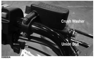
5. Fill the master cylinder with DOT 4 brake fluid; then bleed the system (see Periodic Mainte-nance/Tune-Up - Hydraulic Brake Systems).
