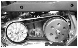
4. Remove the nut securing the movable drive face; then remove the face. Account for the stepped washer and spacer.
