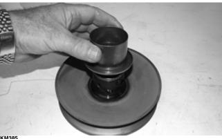
5. Remove four pins and bushings from the fixed face hub; then remove the movable face.
