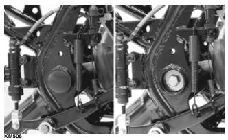
9. From the left side, remove the pivot lock nut using Pivot Lock Nut Wrench; then remove the left pivot adjusting bolt.
