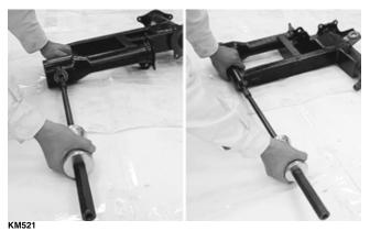
2. Drive in new pivot bearings until fully seated; then install new dust seals.
