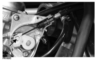
4. Place the throttle actuator cover into position on the carburetor; then secure with the screw.
