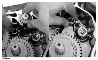
10. Remove the countershaft and driveshaft as an assembly.
