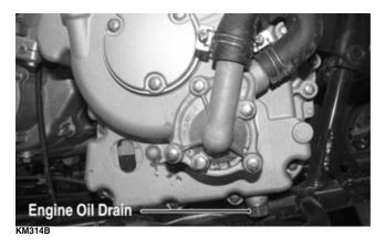
4. Remove the screen/filter cap from the bottom of the engine and drain the oil into a drain pan. Account for a spring, O-ring, and screen/filter. Discard the O-ring.
