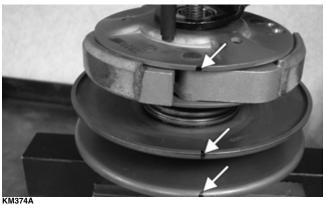
2. Secure the centrifugal clutch with the spring compressor; then remove the drive plate nut.
