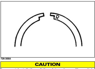
Incorrect installation of the piston rings will result in engine damage.
