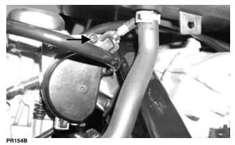
6. Remove the throttle cable from the actuator arm.
