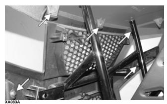
2. Install both headlights assemblies; then connect each connector to the main wire harness connectors. Secure each connector to the frame.
