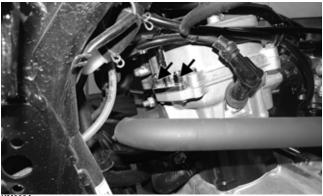
4. Remove the cap screws securing the cylinder head cover. Account for the O-ring.
