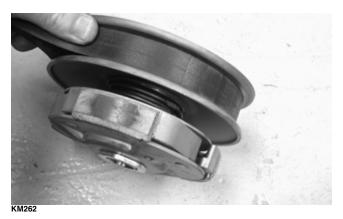
2. Install the centrifugal clutch housing onto the driven shaft; then install the splined bushing and secure with the driven pulley retaining nut. Tighten to 40 ft-lb.
