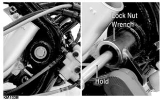
9. Install the shock absorber using the existing hardware and tighten to 29 ft-lb; then install the brakeline hose clamp on the swing arm and tighten securely.
