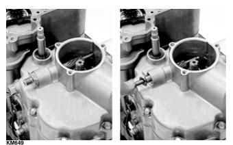
5. Using a Spanner Wrench to hold the centrifugal clutch housing, remove the nut securing the second-ary drive bevel gear to the driveshaft.
