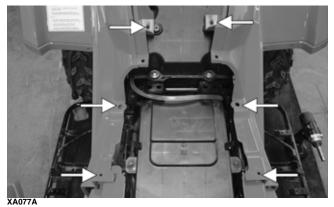
4. Clamp and pinch off the fuel inlet hose to the carburetor. Remove the two fasteners securing the gas tank valve to the gas tank mount. Slide the fuel filter off its mount.
