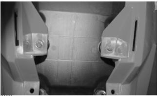
8. Remove the two self-tapping screws securing the inlet of the CVT intake tube to the front body panel.
