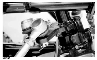
5. Remove the cotter pin and slotted nut from the lower end of the steering post; then remove the upper steering shaft support block. Account for a cable guide, two steering support blocks, and the upper steering post bushing.
