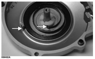
6. Install the ratchets making sure the ends are properly oriented on the reel.
