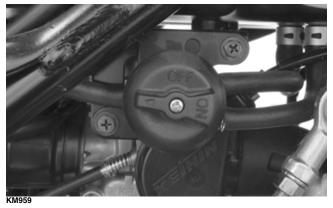
4. Remove the choke assembly from the carburetor leaving the choke cable attached to the choke plunger.
