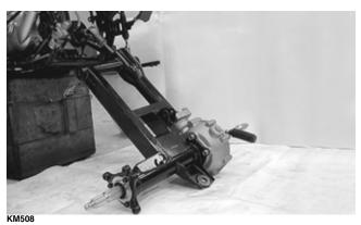
11. Disengage the universal joint from the transmission output shaft splines and set the driveshaft aside.
