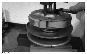
7. Using a suitable holding fixture, tighten the drive plate nut (coated with red Loctite #271) to 43 ft-lb.
