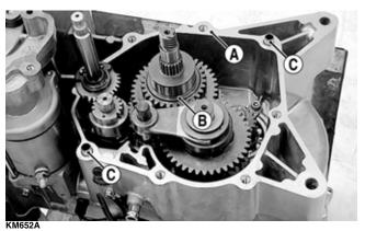
7. Remove the shift shaft; then remove plug, seal/washer, spring, and shift cam stopper ball.
