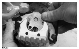
C. Install new brake pads; then install the two brake pad alignment pins.
