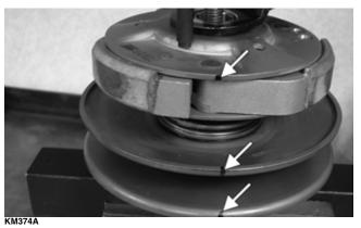
3. Install the pins and spacers into the fixed face hub; then pack the cam slots in the movable face with multi-purpose grease.
