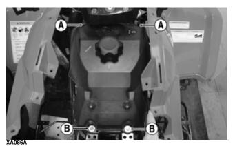
7. Disconnect the fuel level sensor connector; then remove the gas tank.
