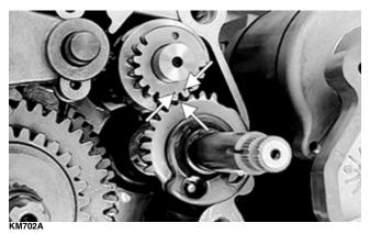
15. Install the two alignment pins, gasket, and transmission case cover and secure with eight cap screws. Tighten in a crisscross pattern to 20 ft-lb.
