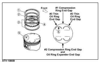
2. Install the compression rings (1 and 2) so the letter on the top surface of each ring faces the dome of the piston. Rotate the rings until the ring end gaps are on directly opposite sides of the piston according to the illustration.
