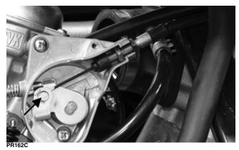
7. Loosen the outer jam nut securing the throttle cable to the carburetor body; then route the cable out of the way.
