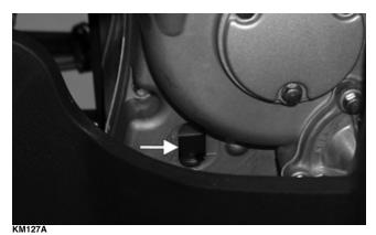
11. Inspect the area around the screen/filter cap for leaks.
