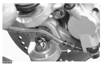
5. Remove the hub assembly; then remove the disc cover.
