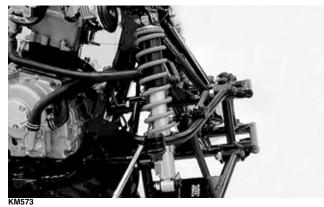
7. Remove the brake hose clamp from the A-arm; then remove the cotter pins and slotted nuts securing the upper and lower ball joints.
