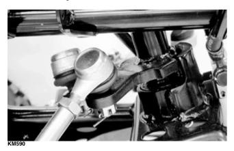
5. Install the handlebar and tighten the clamp cap screws to 18 ft-lb making sure to tighten the front cap screws first.
