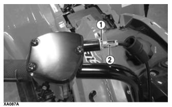
2. Turn the adjuster until the throttle cable has proper free-play of 1-4 mm (1/16-3/16 in.) at the lever.
