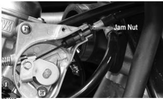
3. Connect the throttle cable to the actuator arm.
