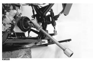
12. Remove the eight cap screws securing the swing arm to the final drive gear case.
