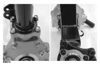
13. Support the swing arm from the right side; then using a rubber mallet, drive the axle shaft from the swing arm tube. Account for two O-rings.
