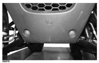
4. From within the front body panel, remove the remaining five cap screws securing the front fascia to the front body panel. Remove the fascia.
