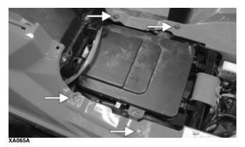
2. Secure the two cap screws securing the lower fascia to the front bumper; then from within the front bumper assembly, secure the additional two caps screws to the frame. Tighten the cap screws from step 1.
