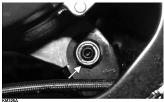
17. Swing the rear of the engine/transmission to the left; then slide the engine out of the left side of the frame.
