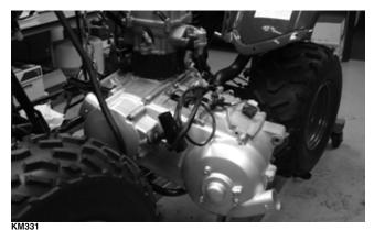
2. Lifting the front of the engine/transmission, move the assembly forward sufficiently to clear the rear engine mounts; then engage the secondary bevel driveshaft into the universal joint splines.
