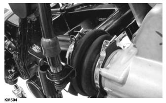
7. Remove the clamp securing the brakeline hose to the swing arm; then remove the lower rear shock absorber mounting nut and bolt.
