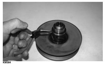
4. Install the spring seat over the hub and movable face hub.
