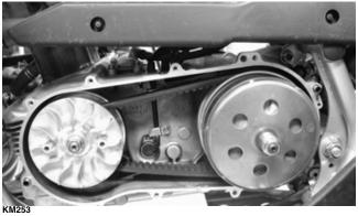
3. Using a suitable holder to prevent the drive pulley from turning, remove the drive face nut and starter ratchet; then remove the drive pulley face.
