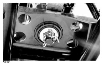
4. Place the inner tie rod ends into the steering post arm and tighten the slotted nuts to 15 ft-lb; then install new cotter pins.
