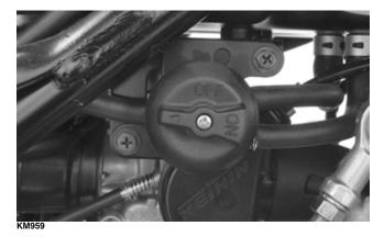
In the OFF position, the valve will not allow gasoline to flow to the carburetor. In the ON position (the normal operating position), gasoline will flow from the tank to the carburetor. In this position, 4.54 L (1.2 U.S. gal.) will remain in the tank as a reserve quantity. Moving the valve to the RES position will allow the operator to use the remaining gasoline in the tank. When turning the valve to any of the three positions, make sure the indicator is pointed directly at the position desired.
