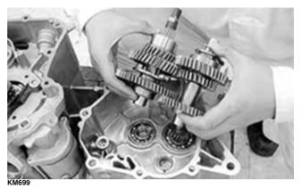
11. Install the low/reverse shift fork into the low/reverse clutch dog; then install the shift cam into the transmission case and engage the shift fork pawl in the appropriate shift cam groove.
