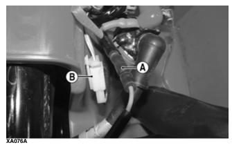
6. Place each tail light/brake light assembly into place and secure with the cap screws. Connect each wire connector to the main harness; then secure to the frame.
