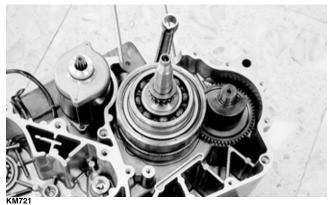
2. Remove the balancer shaft from the left crankcase half.
