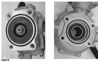
3. Inspect all splines and hubs for excessive wear, chips, cracks, or distortion.
