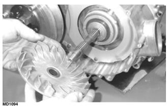
2. As noted during disassembling, place each roller into each valley of the movable drive sheave. With the dampers installed onto the sheave plate, install the sheave plate into the movable drive sheave.
