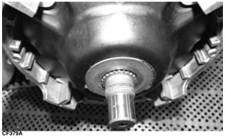
■NOTE: At this point with both the 570 and 700EPS, the cap screw can be removed from the driven pulley.
