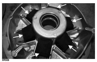
4. Compress the outer portion of the drive clutch toward the sheaves; then install the nut on the end of the drive clutch. Tighten to 79.6 ft-lb.
