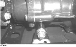
17. Remove the upper differential mounting cap screws. Account for the spacer.
