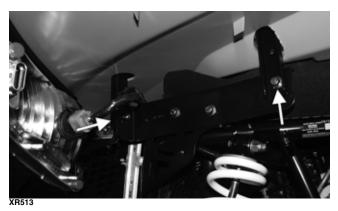
10. Remove the four Torx-head screws securing the fascia to the front bumper.
