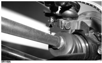
4. Apply a small amount of grease to the hub splines.
