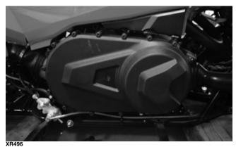
2. Remove the belt; then with the Drive Clutch Spanner Wrench to secure the drive clutch, remove the bolt securing the drive clutch; then insert the Drive Clutch Puller and remove drive clutch.
