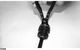
2. Place the white-striped end of the CV joint into a
