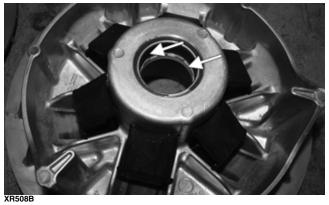
3. Install the pucks; then position the movable sheave onto the drive clutch assembly.
