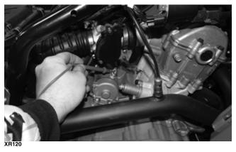
■NOTE: If the meter showed correct voltage but the starter motor did not operate or operated slowly, troubleshoot all starting system components before replacing the starter motor.
