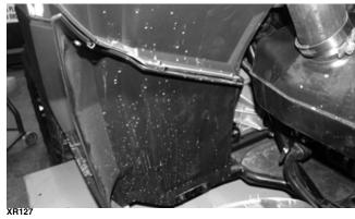
3. Remove the hose clamp securing the gas tank to the gas tank hose. Account for the hose clamp.
