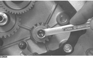
6. Install the shift cam stopper, spring, and two washers (thick washer closest to the nut); then coat the threads on the mounting stud with red Loctite #271 and install the nut. Tighten to 8 ft-lb.
