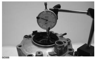
Zero the dial indicator; then push the ring gear toward the dial indicator and release. End-play should be 0.004-0.008 in.
