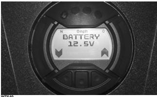
Display: System DC voltage. DTC: P0562, P0563, P2531, P2532
