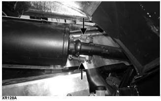
5. Remove the muffler and account for a GRAFOIL seal.
