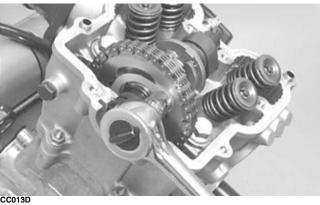
8. While holding the chain, slide the sprocket and camshaft out of the cylinder head.
