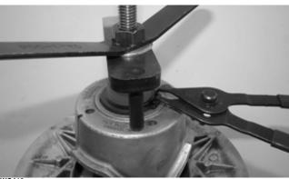
9. Turn the wing nut counterclockwise slowly allowing the cam to contact the snap ring; then loosen slightly and tap the cam with a plastic mallet to ensure the snap ring is securely seated.
