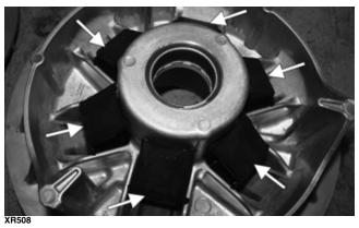
Check the internal bushing of the movable drive sheave. Replace as necessary. Check the fixed drive sheave internal splines for excessive wear.
