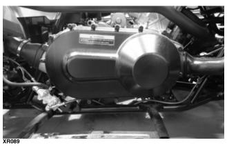
2. Remove the nut securing the movable drive face; then remove the face. Account for a spacer.
