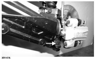
3. Install the tie rod end and secure with the nut. Tighten to 30 ft-lb; then install a new cotter pin and spread the pin.
