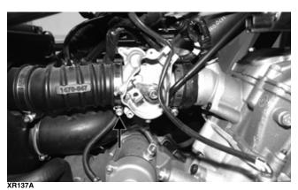
■NOTE: Removing the air filter housing boot from the filter housing will aid in removing.
