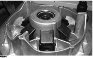
Note the puck orientation and locations; then remove the pucks. Check for abnormal wear. If excessively worn, replace as necessary; then remove the movable sheave from the drive clutch assembly.
