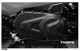
On the 570, remove the nut securing the movable drive face; then remove the face. Account for the flat washer and spacer.
