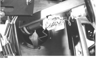
3. Rotate the fuel pump until the match marks align; then install the mounting screws and tighten securely using a crisscross pattern.
