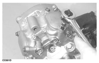
**■NOTE:** Keep the mounting hardware with the covers for assembly purposes or thread them back into the head to keep them separated.
