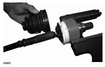
■NOTE: Steps 1-3 can be used to replace the outboard boot.
