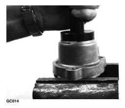
3. Lubricate the input shaft with High-Performance #2 Molybdenum Disulfide Grease packing the boot ribs and splines; then assemble allowing excess grease to freely escape. Slight pressure on the boot will be present during assembly. Secure with new clamps.
