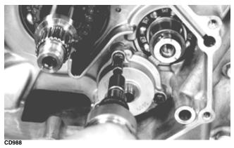
4. Install the oil pump drive gear spacer onto the crank balancer shaft. Grease the pin and insert it into the shaft; then install the drive gear making sure the raised side of the gear is facing toward the inside. Secure the gear with the cap screw (threads coated with red Loctite #271) and the washer. Tighten the cap screw to 63 ft-lb.
