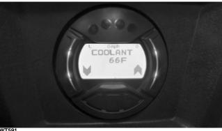
Display: Engine coolant temperature as measured by the ECT
