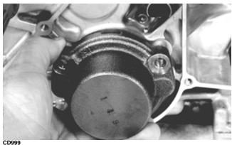
8. Remove the snap ring securing the oil pump driven gear (A); then remove the gear, noting the direction of the sides of the gear for installation purposes. Account for a pin and a washer.
