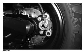
■NOTE: During the bleeding procedure, watch the reservoir very closely to make sure there is always a sufficient amount of brake fluid. If low, refill the reservoir before the bleeding procedure is continued. Failure to maintain a sufficient amount of fluid in the reservoir will result in air in the system.
