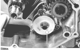
9. Using an impact driver, remove the three Torx-head screws securing the oil pump; then remove the pump.
