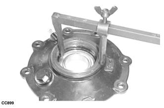
■NOTE: Prior to installing the seal, apply High-Performance #2 Molybdenum Disulfide Grease to the seal outside diameter.
