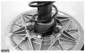
4. Place the cam over the spring and align the spring tip to the previously marked anchor hole.
