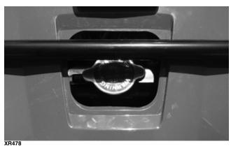
3. Add coolant as necessary; then install the radiator cap and access plug.
