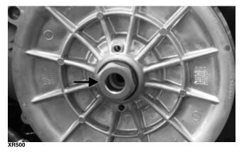
11. Spread the faces of the driven clutch by threading the cap screw from the tool kit into the boss of the driven fixed face; then tighten the cap screw until the V-belt drops into the driven pulley.
