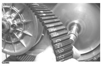
■NOTE: The arrows on the V-belt should point in the direction of rotation.
