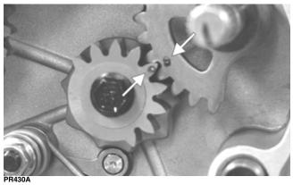
15. Remove the gear shift cam plate and account for a washer; then remove the cam stopper and cam stopper spring. Account for two washers.
