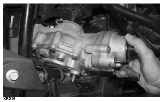
2. Align the four holes in the output flange and install the four cap screws (coated with blue Loctite #243). Tighten to 20 ft-lb. Pull the rubber boot over the output flange and input shaft. Be sure to align the oil rings over the recess.
