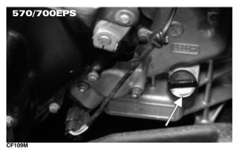
3. Remove the drain plug from the bottom of the engine and drain the oil into a drain pan. Account for and discard the drain plug gasket.
