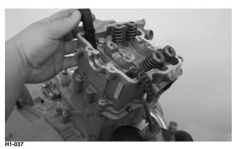
10. Remove the five nuts securing the cylinder head to the cylinder.
