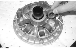
3. Check the internal bushing of the movable drive sheave and surface of the spacer. Replace as necessary. Check the fixed drive sheave internal splines for excessive wear. Check for any broken cooling fins and replace as necessary.
