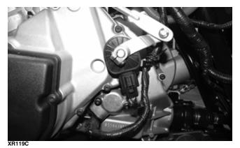
1. Disconnect the gear position switch connector; then using a multimeter, test the switch in each position as follows. Resistance must be less than 1 ohm for all tests.
