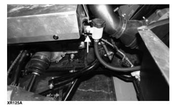
■NOTE: Using an appropriate tool, pry the tab of the master cylinder mounting bracket from the gas tank.
