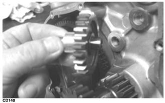
12. Remove the snap ring securing the water pump drive gear; then remove the gear noting the direction of the sides of the gear for installing purposes. Account for the drive gear alignment pin.
