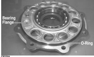
5. Making sure the O-ring is properly positioned on the differential housing cover assembly, install the cover with existing cap screws (coated with green Loctite #609). Tighten the cap screws evenly to 23 ft-lb (existing housing) or 28 ft-lb (new housing).
