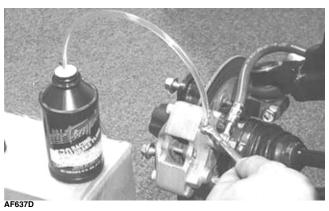
2. Place an absorbent towel around the connection to absorb brake fluid. Remove the banjo-fitting from the master cylinder. Account for two crush washers and a banjo-fitting bolt.
