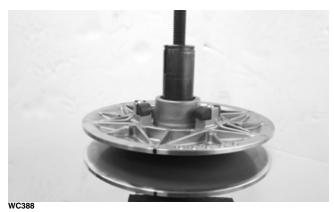
3. Install the spring over the hub of the movable driven sheave engaging the spring into the previously marked spring anchor hole.
