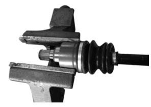
3. To disengage the axle from the CV joint, sharply pull back on the axle; then slide the boot off of the axle.
