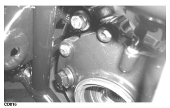
18. Remove the four cap screws securing the output flange; then shift the differential assembly forward enough to disengage the output flange assembly.
