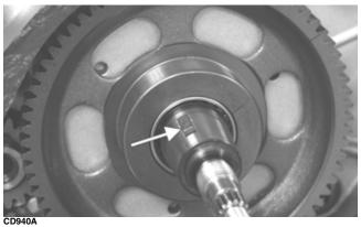
11. Remove the two starter gears from the crankcase noting the direction of the gears for installing purposes; then remove the two starter gear shafts.
