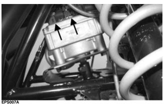
10. Remove four cap screws securing the EPS housing to the frame; then lift the assembly upward sufficiently to disengage the lower coupler and remove from the left side.
