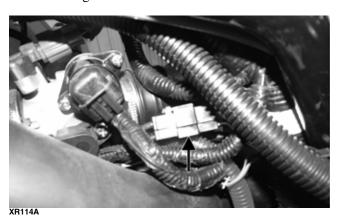
■NOTE: Test the connector that comes from the engine.
