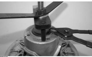
9. Turn the wing nut counterclockwise slowly allowing the cam to contact the snap ring; then loosen slightly and tap the cam with a plastic mallet to ensure the snap ring is securely seated.
