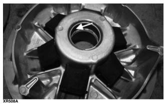
4. Remove the spring (E); then the washer (D); then the cup (C) with washer; then the plastic spacer (B); then the bearing (A). Check for any broken/excessively worn parts and replace as necessary.
