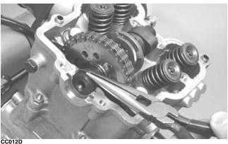
7. Bend the washer tabs down and remove the two cap screws securing the sprocket to the camshaft; then drop the sprocket off the camshaft.
