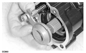
8. Place the input shaft assembly onto the gear case housing; then secure with the existing cap screws. Tighten to 23 ft-lb (existing housing) or 28 ft-lb (new housing).
