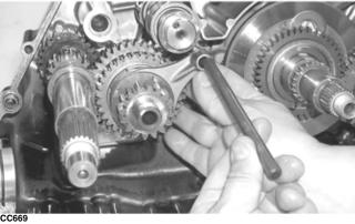
9. Install the reverse idler gear assembly noting the positioning of the two washers, gear, bushing, and shaft.
