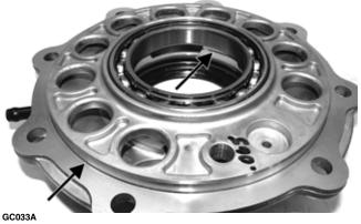
4. Install the existing shim or a 1.6 mm shim on the cover side of the ring gear; then place the assembled gear case cover onto the gear case and secure with three cap screws. Tighten evenly using a crisscross pattern.
