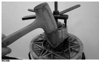
10. Remove the wing nut, compression yoke, and centering bushing; then remove the driven pulley assembly from the Clutch Spring Compressor.
