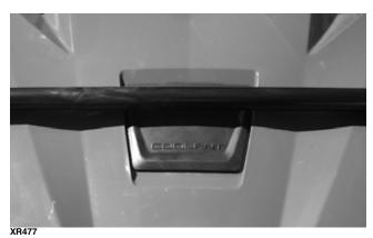
2. Carefully rotate the radiator cap counterclockwise to release pressure; then remove the cap.
