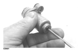
■NOTE: The adjuster shaft will be drawn into the tensioner as the adjuster screw is rotated clockwise. The adjuster shaft tension will be released in step 25.
