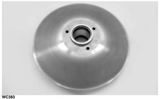
2. Inspect the cam shoes on the movable driven sheave for chipping, excessive scoring, or general condition.
