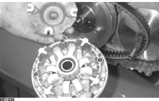
2. Note the roller locations; then remove the rollers. Check for flat spots or abnormal wear. Measure the outside diameter; standard measurement is 30 mm. If excessively worn, replace as necessary.
