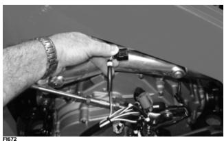
3. Using a multimeter, connect the black tester lead to the black socket (GND) on the analyzer and the red tester lead to the white socket (VAR); then select the DC Voltage position. With the vehicle off, the gauge should read 0.58-0.62 and at Wide-Open Throttle it should read up to approximately 3.7.
