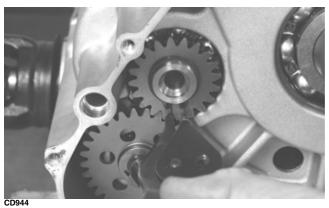
13. Remove the snap ring securing the water pump driven gear; then remove the gear noting the direction of the sides of the gear for installing purposes. Account for the driven gear alignment pin.
