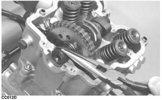
22. Install the cylinder head plug in the cylinder head with the open end facing downward and toward the inside.
