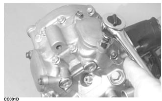
33. If removed, install the spark plug. Tighten securely.
