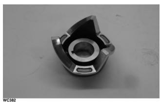
4. Inspect the key and keyways in the cam and fixed driven sheave for excessive wear.
