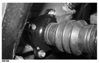
19. Place the differential on its left side; then remove it from the frame.
