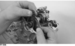
9. Remove the cap screw securing the chain tensioner (account for a washer); then remove the tensioner.
