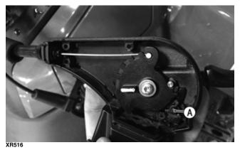
3. Remove the cable from the shift switch; then remove the cable from the vehicle taking note of routing and any fastening points of the cable.
