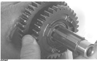
4. Install the outer reverse driven washer; then secure the reverse driven gear assembly with a snap ring.
