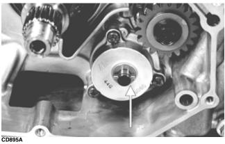
13. Using an impact driver, remove the three Torx-head screws securing the oil pump; then remove the pump.
