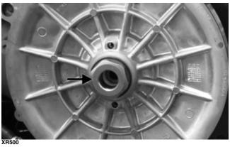
4. Remove the cap screws securing the inside clutch cover. Note the location of the different-length cap screws for installing purposes. Using a rubber mallet, carefully remove the cover. Account for two alignment pins.
