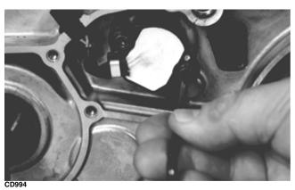
2. Install the secondary shaft bearing housing making sure the two alignment pins are properly positioned. Tighten the new "patch-lock" cap screws to 28 ft-lb.
