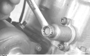
26. Loosen the four adjuster screw jam nuts; then loosen the four adjuster screws on the rocker arms in the valve cover.
