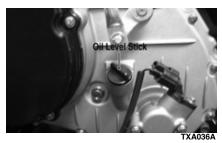
There is an oil level stick for checking the engine oil level. To check the oil level, use the following procedure:
