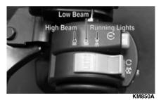
Use the headlight HI/LO switch to select the high or low headlight beam when the ignition switch is in the LIGHTS position. When the switch is in the HI position, the high beam will illuminate. When the switch is in the LO position, the low beam will illuminate. When the switch is in the Running Light position, the taillights and running lights will illuminate.
