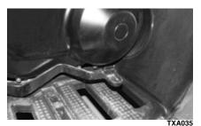
Pressing the rear foot brake downward will apply the brake to the rear wheels.
