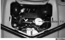
5. Install the radiator cap and access panel.
