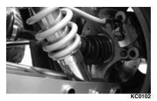
■ NOTE: Before attempting to adjust suspension, clean dirt and debris from the sleeve and remove load from the suspension; then use the spanner wrench to adjust the sleeve to the desired position.
