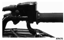
Control engine RPM with the position of the throttle lever. Operate this lever with the thumb. Pushing it forward increases engine RPM and allowing it to retract decreases engine RPM.
