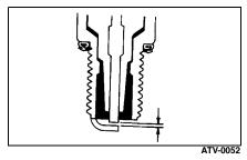
When installing the spark plug, be sure to tighten it securely. A new spark plug should be tightened 1/2 turn once the washer contacts the cylinder head. A used spark plug should be tightened 1/8-1/4 turn once the washer contacts the cylinder head.
