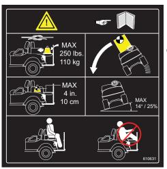
LOAD WITH HIGH CENTER OF GRAVITY COULD CAUSE TIP OVER
