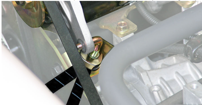
Fig. 11 Adjusting the Belt Tension
